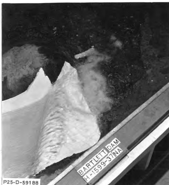
A. Recommended concrete fill.
