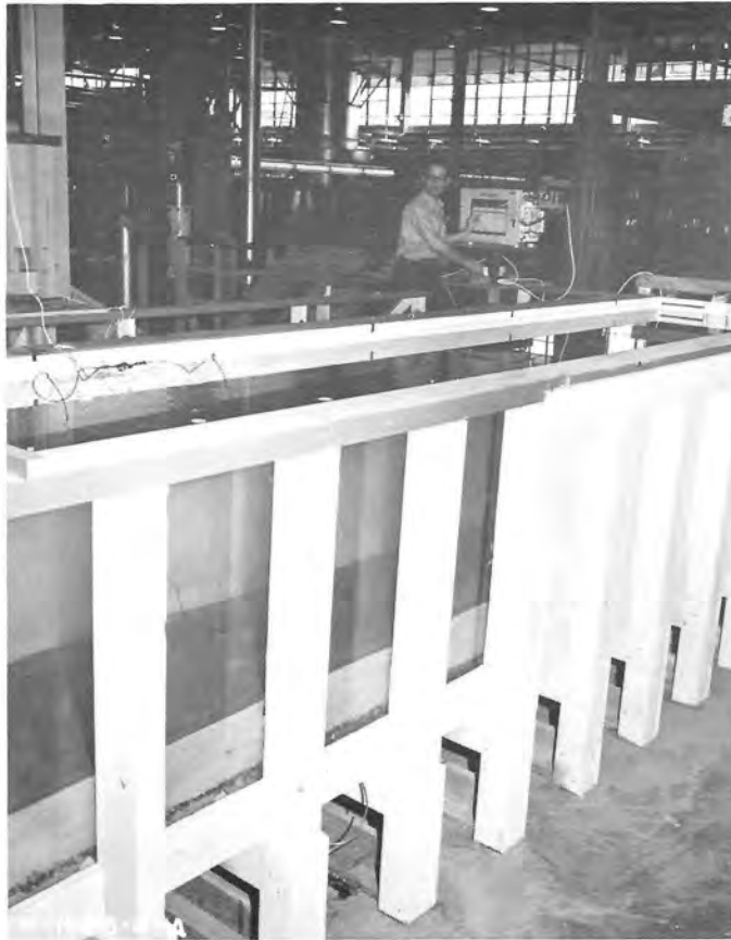
Figure 12. Seepage loss detection by electrical logging techniques was studied in a wooden flume thereby reducing the possibility of interference of measurements by magnetic fields.
