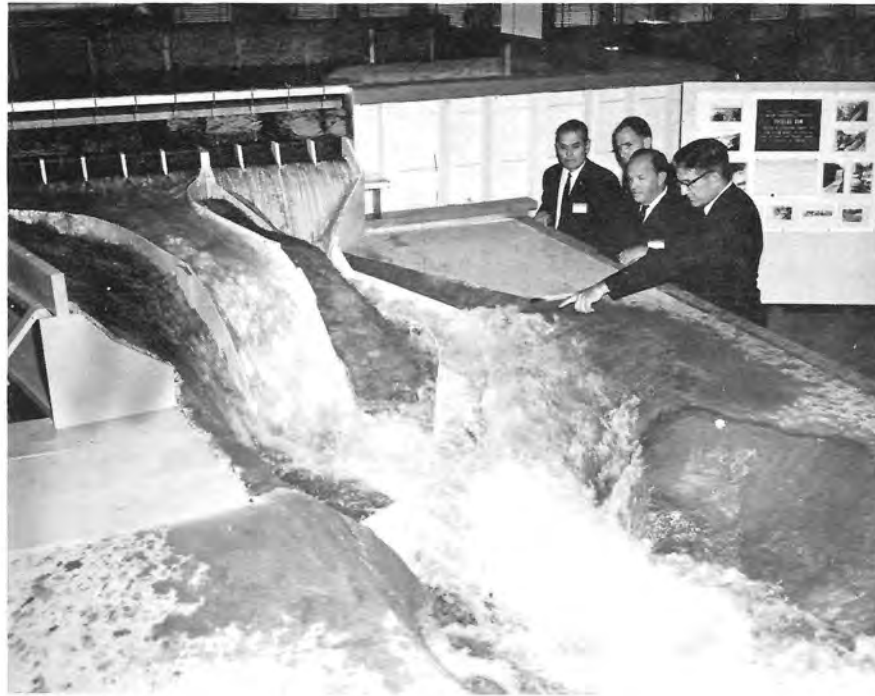
Figure 10. A 1:36 scale hydraulic model of the Patillas Dam spillway is being studied to improve the capacity and safety of the structure.
