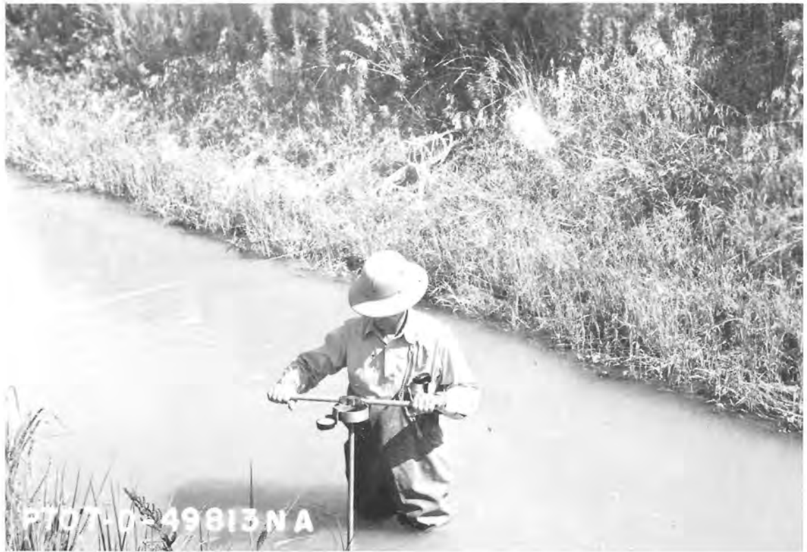
Figure 13. Hydraulic tractive force measurements were made in three test reaches of the Farwell Main Canal. A vane shear measurement of the canal bottom soil is being made.
