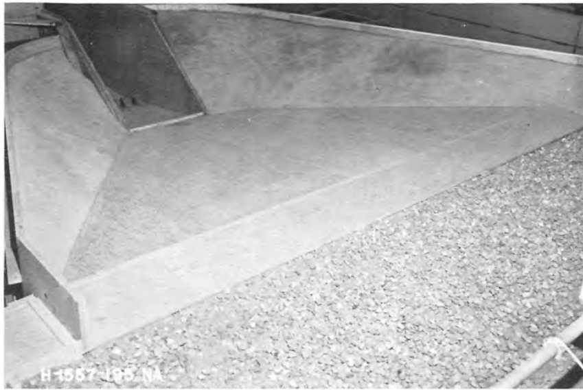
Figure 4. Model simulation of paved downstream channel, Navajo Dam outlet works.
