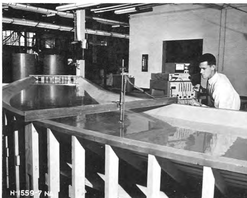
Figure 14. Boundary shear distribution measurements are being made on a rigid boundary trapezoidal laboratory canal.
