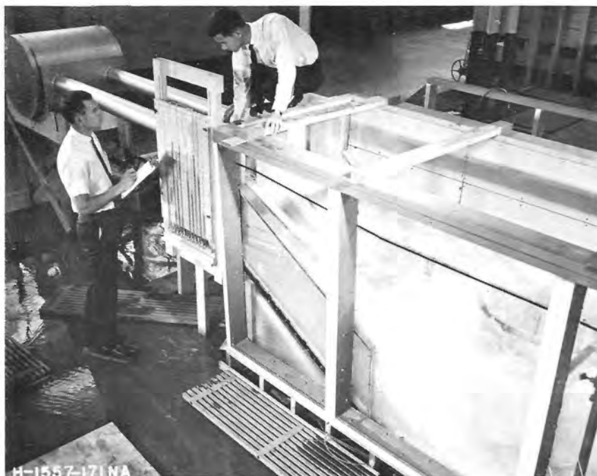
Figure 15. Measurements of dynamic pressures and vibrations are being made in a hydraulic model of a hollow-jet valve stilling basin.
