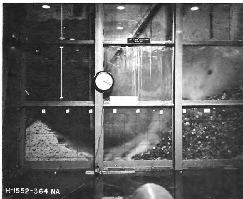
Figure 1. A full-scale sectional model was used to develop a technique of removing sediment from the spawning gravel in the Tehama-Colusa Canal. Fine sediment is washed from the gravel as a baffle gate is moved slowly upstream.
