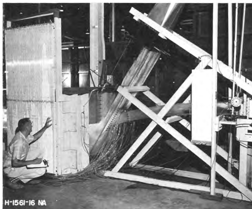
Figure 7. Hydraulic model (1:16.7 scale) of a single upper tier outlet and junction with spillway, Folsom Dam. Studies are aimed at alleviation of negative pressures at the juncture.
