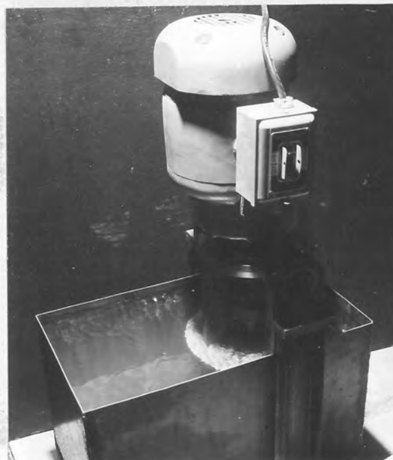
D. Apparatus operating at 780 rpm. Note slight turbulence on the water surface.
