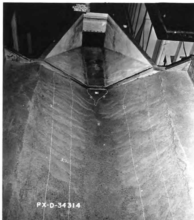
A. Scour after 1 hour. Q = 3.1 , V_p = 4.0 , canal depth = 1.3D .
