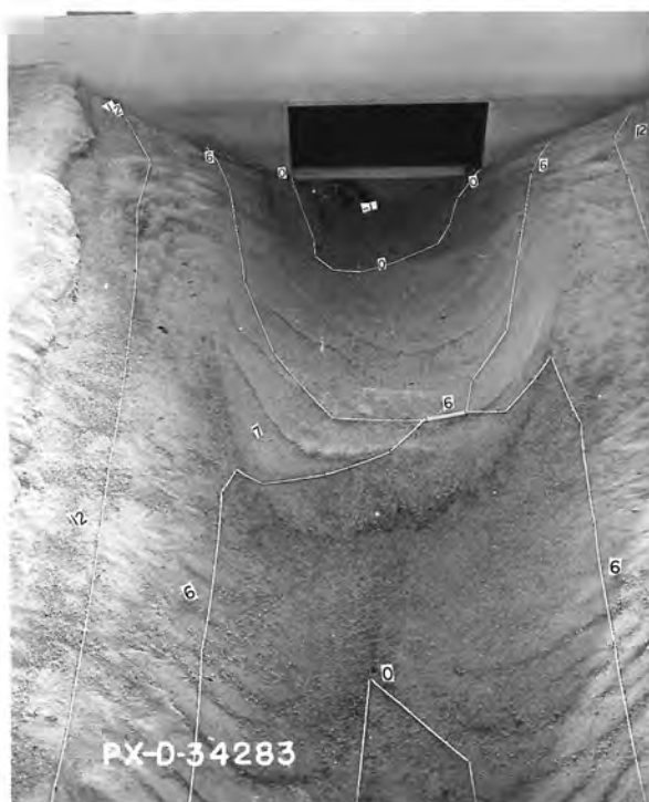
B. Scour after 2 hours operation. V_p = 4.0 f/s, canal depth 1.25D .
