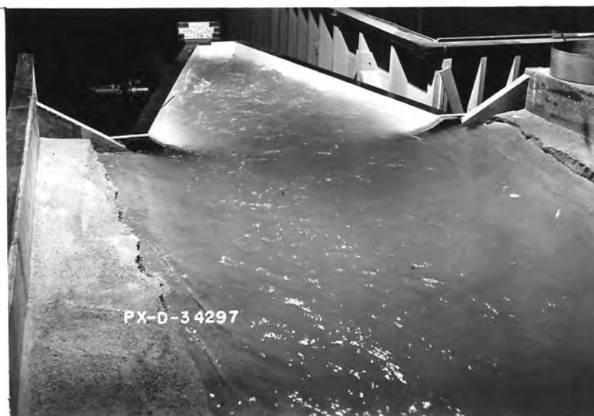
A. The water surface is somewhat rough. Q = 4.7 , V_p = 6.0 , depth = 1.3D.
