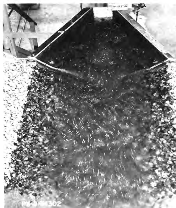
B. Flow conditions. Q = 4.7 , V_p = 6 f/s. Scour occurs at end of riprap.
