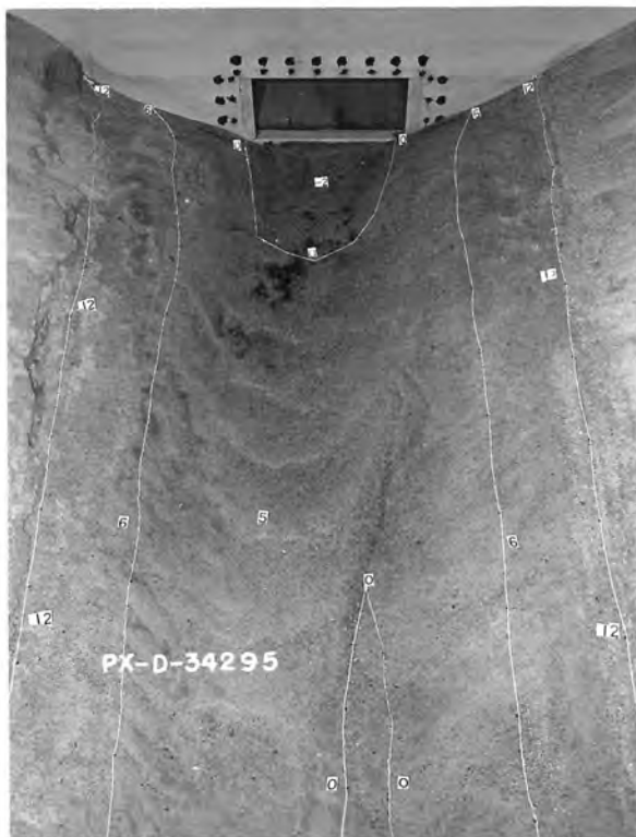
B. Scour after 1 hour operation. Canal depth = 1.00D .
