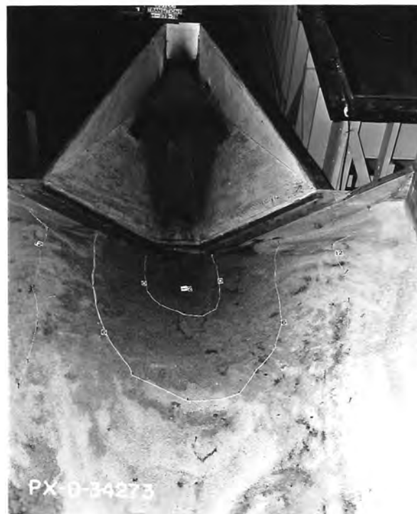
C. Scour after 45 minutes operation with hood installed in transition. Q = 4.7 , V_p = 6.0 , depth = 1.3D .
