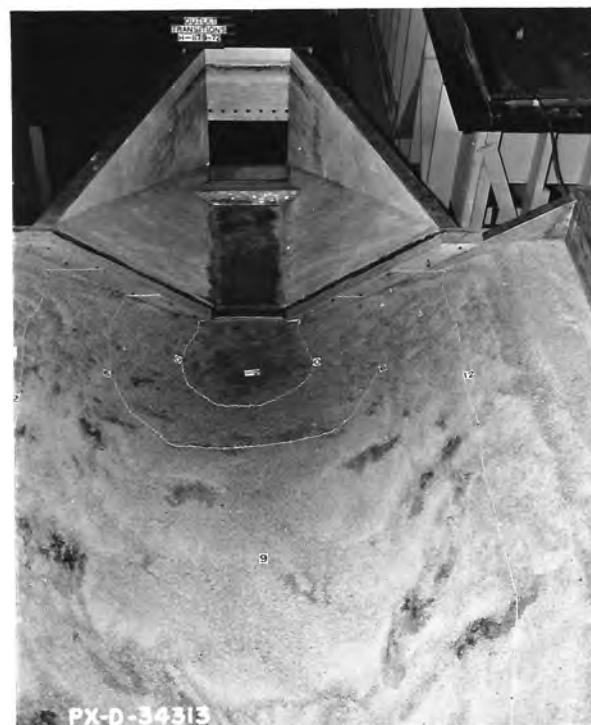
C. Scour after 1 hour operation 3-3/8-inch-high deflector. Q = 4.7 , V_p = 6.0 cfs.
