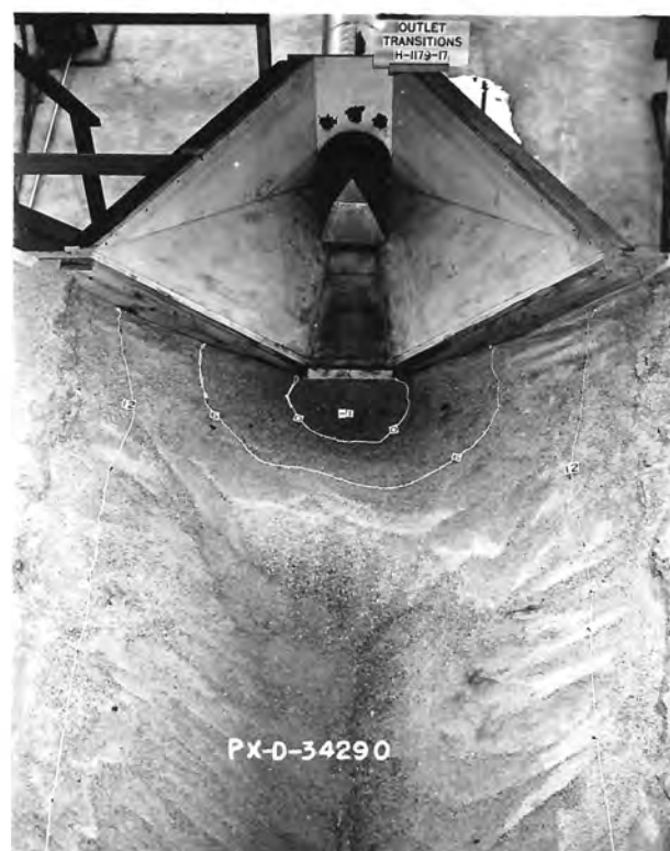
C. Scour 75 minutes operation with hump. Q = 2.4 , V_p = 3.0 , depth = 1.5D .
