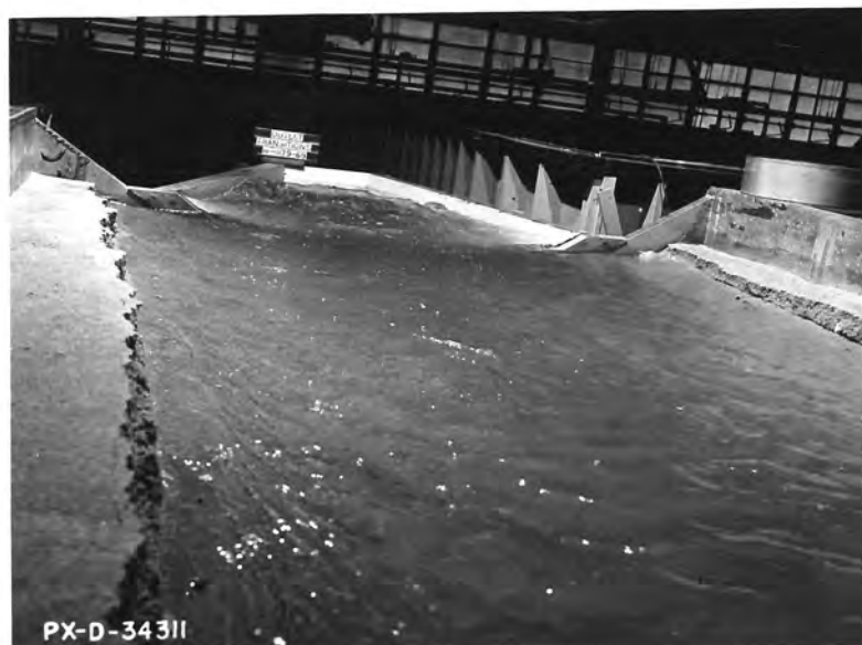
A. A hump occurs in the water surface above the Design 2, hump-like deflector on the floor. Q = 4.7 , V_p = 6.0 , canal depth = 1.3D .
