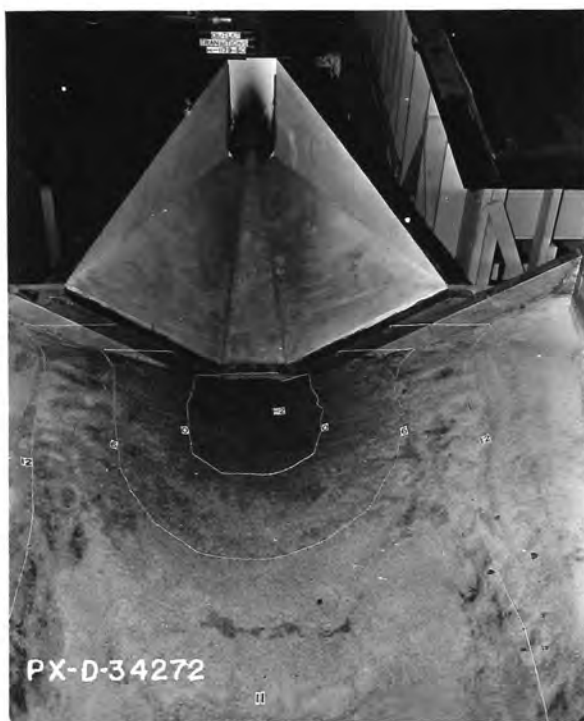
B. Scour after 1 hour operation. Q = 4 . V_p = 6.0 , depth = 1.3D .
