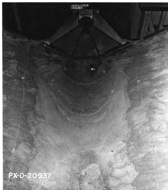
B. Scour after 30 minutes operation each at flow velocities in pipeline of 2, 2.5, and 3 f/s. Depth = 0.8D .
