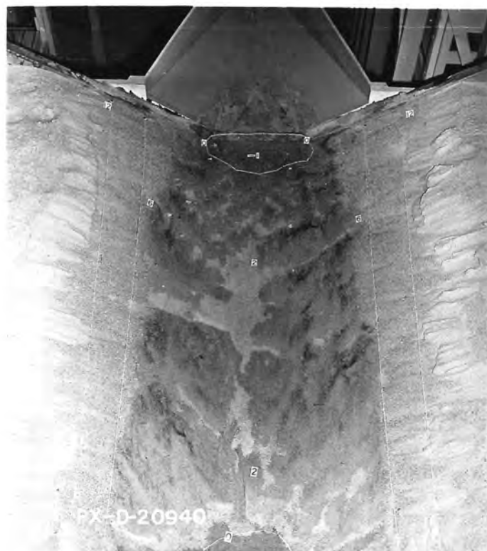
B. Scour after 2-1/2 hours, V_p = 2, 2.5, and 3 \text{ f/s} ; canal depths of 8, 10, and 12 inches. Pipeline on 2:1 slope, depth = 0.8D .
