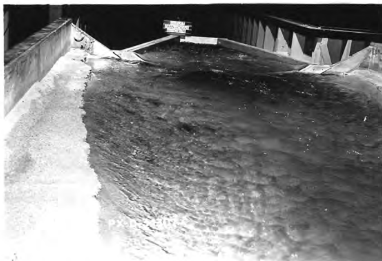
A. Somewhat turbulent water surfaces occur in the transition and canal. Q = 4.7 , V_p = 6.0 , canal depth = 1.3D .
