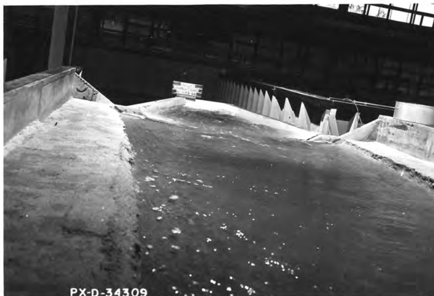
A, Water surface is mildly turbulent in transition, but smooth in canal. Q = 4.7 , V_p = 6.0 , canal depth = 1.3D .
