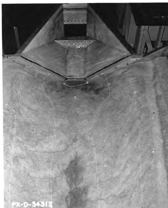
B. Scour after 1 hour operation 6-3/8-inch-high deflector. Q = 4.7 , V_p = 6.0 f/s.
