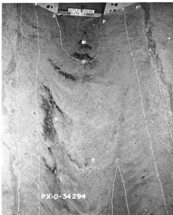
A. Scour after 1 hour operation. Canal depth = 0.83D .
