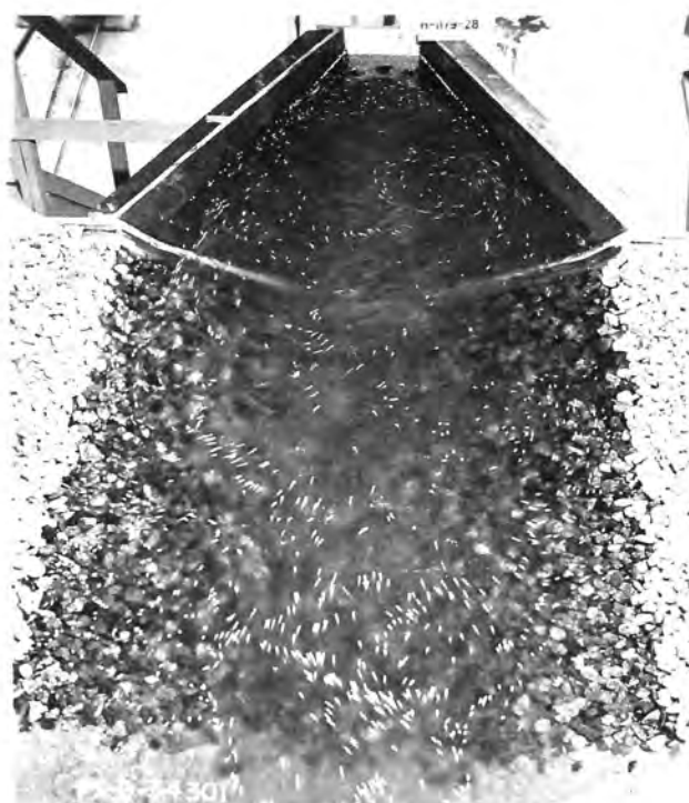
A. Flow conditions. Q = 2.4 , V_p = 3 f/s. Scour was negligible.
