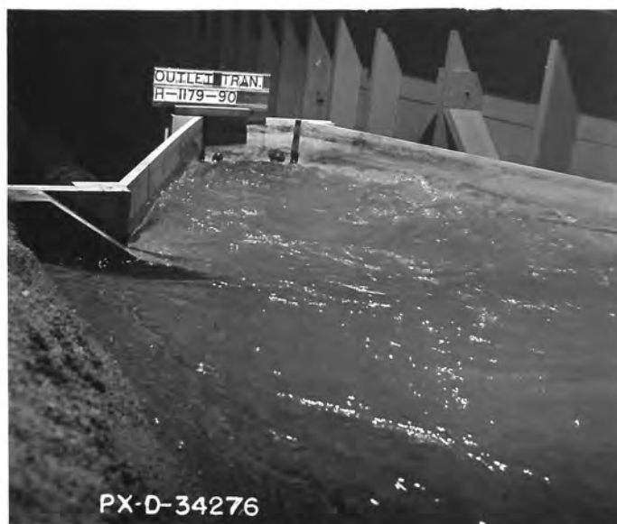
A. Turbulent water surface. Q = 2.4 , V_p = 3.0 , depth = 0.8D .
