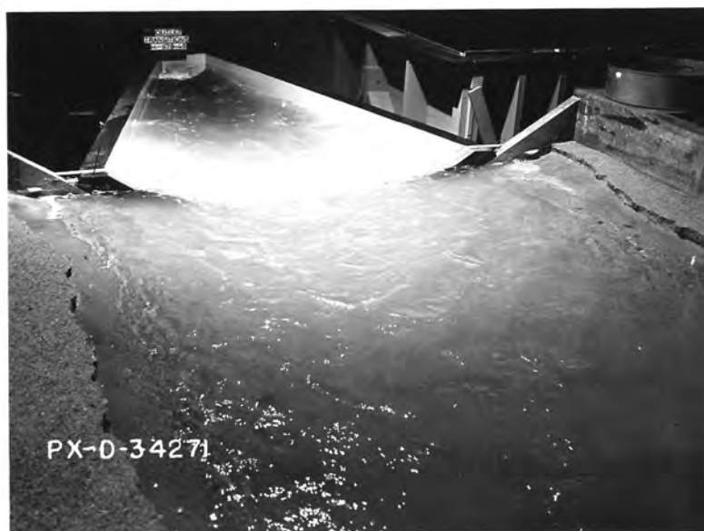
A. The water surface is mildly turbulent. Q = 4.7 cfs, V_p = 6.0 f/s, depth = 1.3D .
