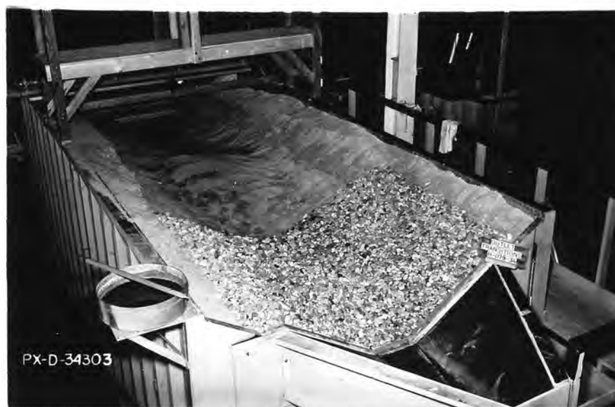
C. Scour after 1 hour at Q = 3.1 cfs, V_p = 4 f/s and 1 hour at Q = 4.7 cfs, V_p = 6 f/s, canal depth = 1.3D .
