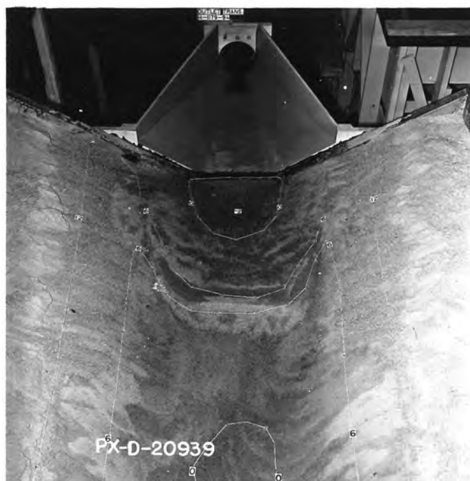
A. Scour after 2-1/2 hours, V_p = 2, 2.5, and 3 \text{ f/s} ; canal depths of 8, 10, and 12 inches. Pipeline horizontal.
