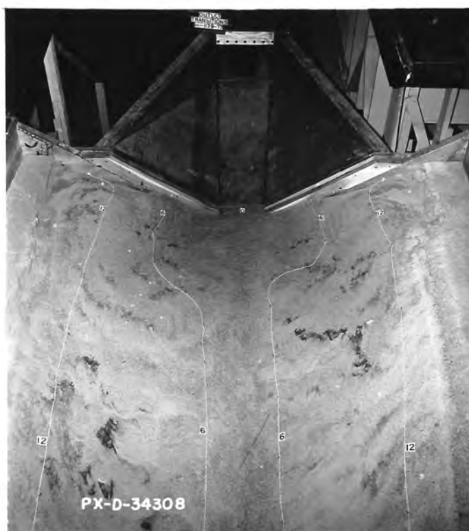
B. Scour after 1 hour operation. Q = 4.7 , V_p = 6.0 , canal depth = 1.3D .
