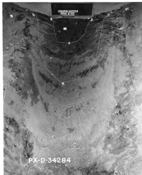
C. Scour after 1 hour operation. V_p = 6.0 f/s, canal depth 1.25D .
