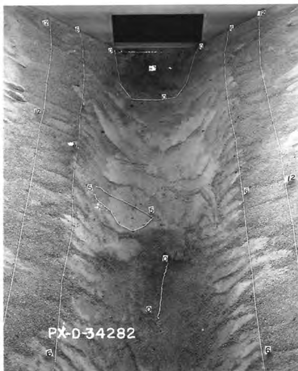
A. Scour after 2 hours operation. Q = 3.1 , V_p = 4.0 , canal depth = 1.0D .
