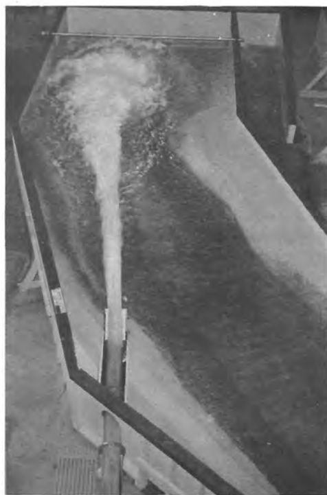
D. 30° flip bucket, with deflector H-1321-99
