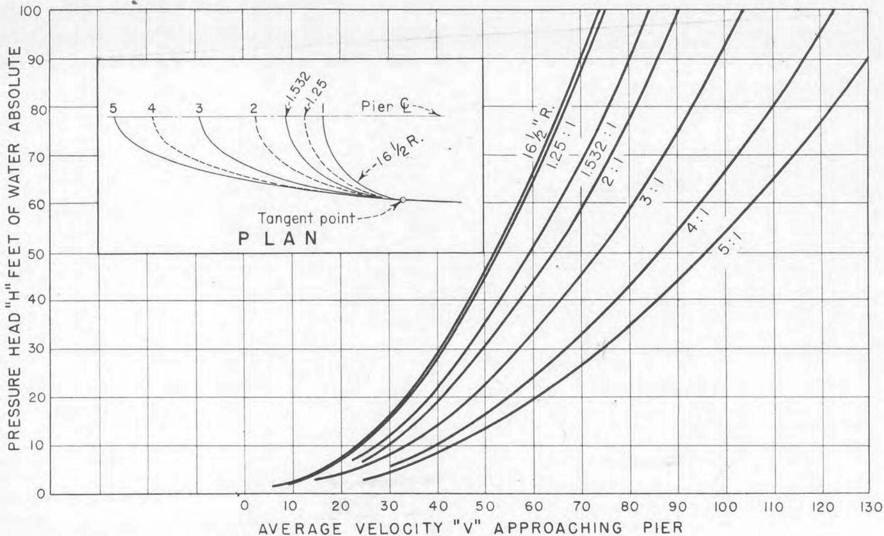
AVERAGE VELOCITY RELATIONSHIP FOR INCIPIENT CAVITATION - ELLIPTICAL PIER NOSE SHAPES
