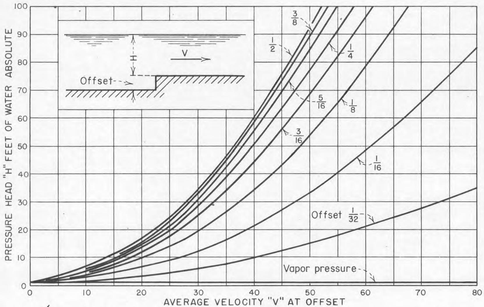
FIGURE 2.6.- HEAD-VELOCITY RELATIONSHIP FOR INCIPIENT CAVITATION—ABRUPT, INTO-THE-FLOW OFFSETS
