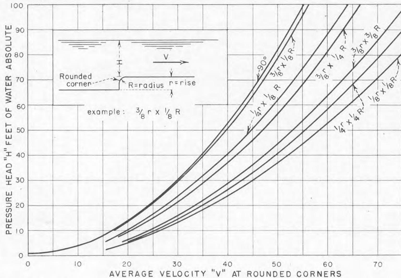
**AVERAGE VELOCITY RELATIONSHIP FOR INCIPIENT CAVITATION - ROUNDED CORNERS**
