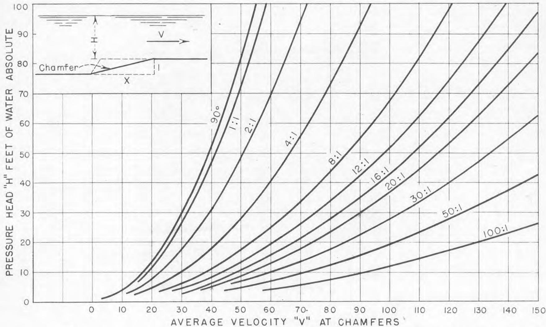
AVERAGE VELOCITY RELATIONSHIP FOR INCIPIENT CAVITATION - INTO THE FLOW CHAMFERS
