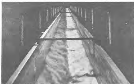
FIG. 2.—AIR ENTRAINMENT CAUSED BY SIDE-WALL EFFECT IN NARROW CHUTES
