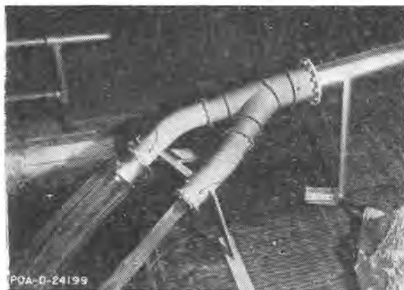
Fig. 12a — United States Outlets Right Outlet Complete Orifice replacing left hollow-jet valve Model scale 1 : 12
