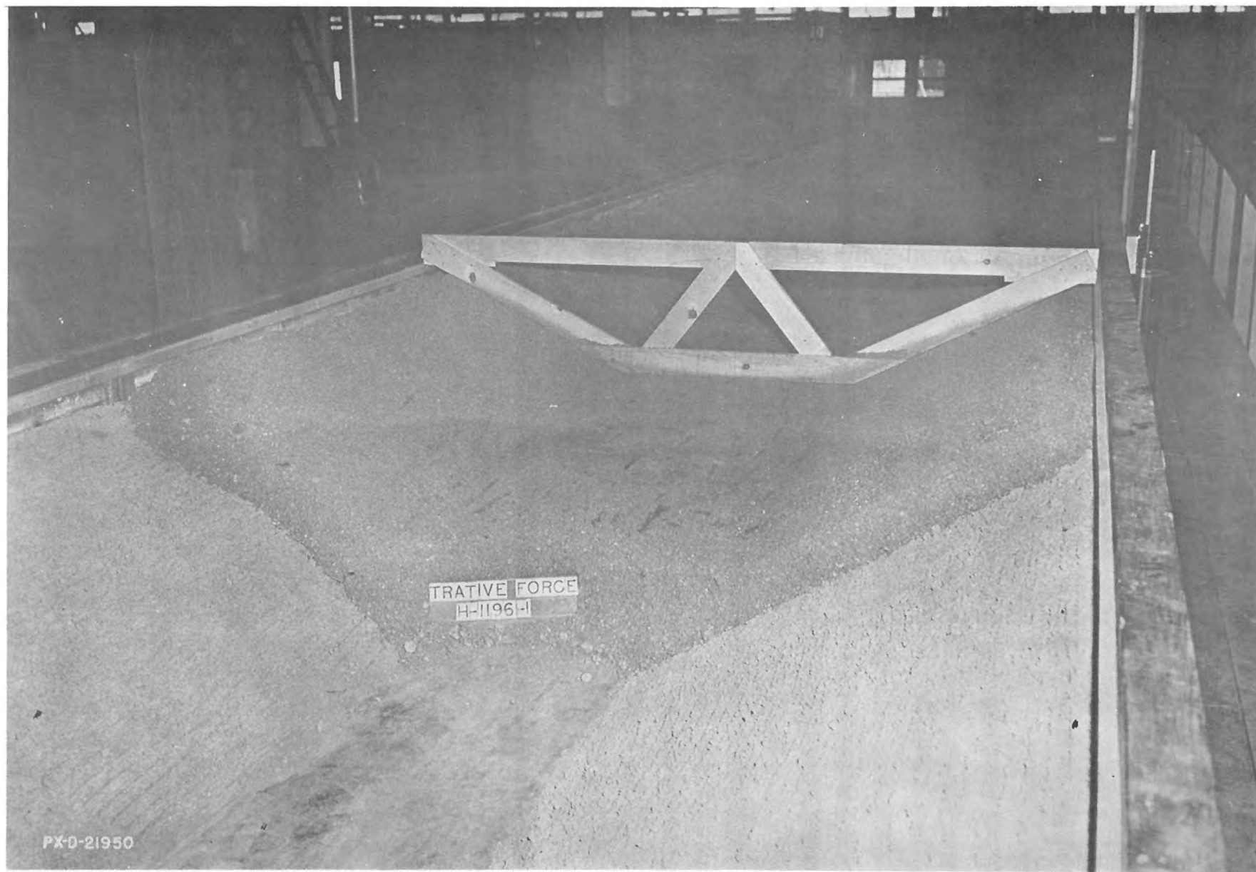
TEMPLATE USED FOR SHAPING CHANNEL
