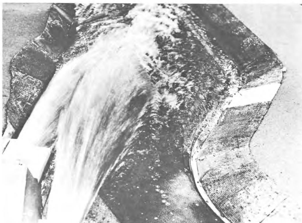
Both Model Tunnels discharging 12,500 cfs each. P-232-D-17060
