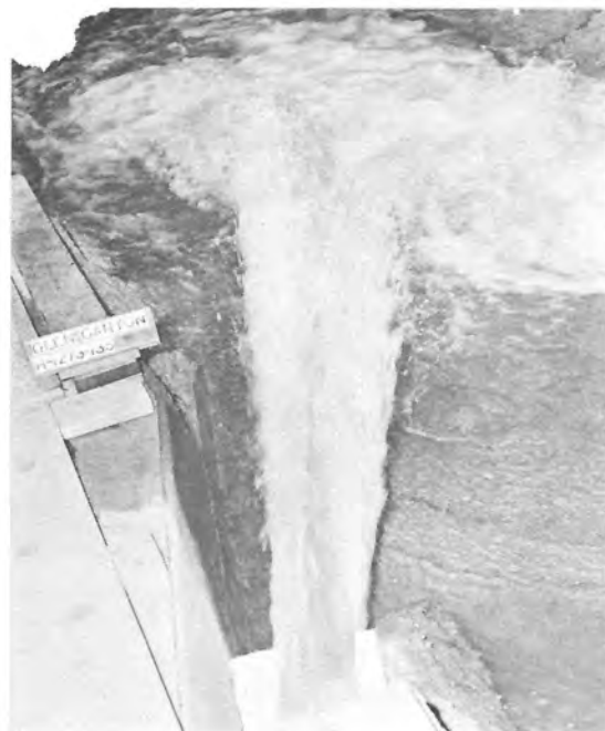
TRANSITION FLIP BUCKET WITH SIDE WALL DEFLECTOR Froude No. = 5.64 P-557-D-17051 & P-557-D-17052
