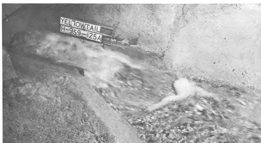
Q = 12,000 cfs Hydraulic jump in Basin P-459-D-17045
