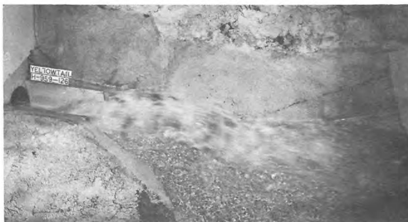
Q = 13,000 cfs, Basin acts as Flip Bucket P-459-D-17046
