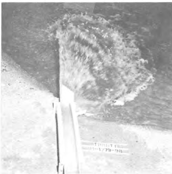
A. DISPERSION TYPE FLIP BUCKET P-208-D-17044
