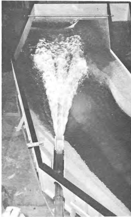
Well dispersed jet at low flows Froude Number = 10.3 P-591-D-17054 & P-591-D-17055
