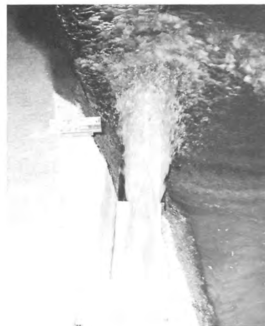
TRANSITION FLIP BUCKET Flow at Froude No. = 5.64 P-557-D-17049 & P-557-D-17050
