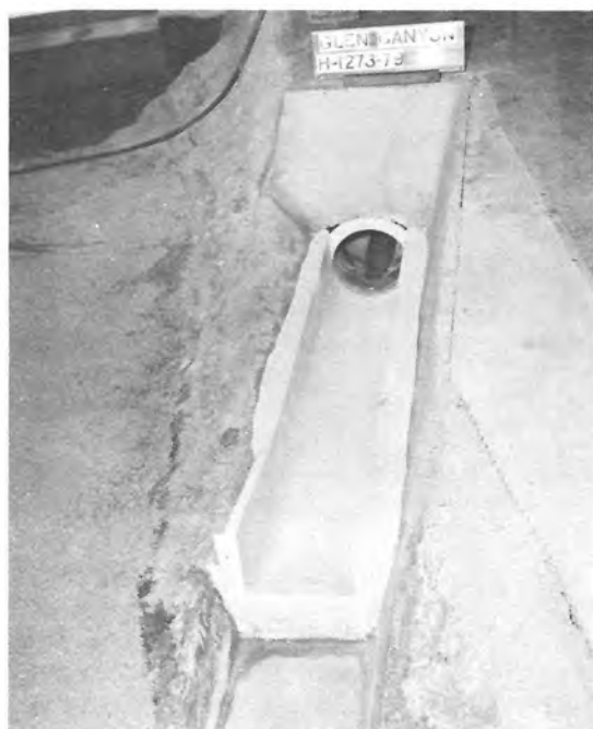
TRANSITION FLIP BUCKET Flow at Froude No. = 5.64 P-557-D-17049 & P-557-D-17050
