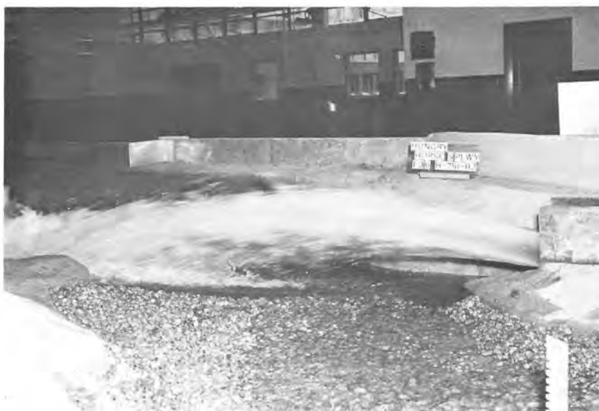
Hungry Horse spillway model discharge = 35,000 cfs P-447-D-17058
