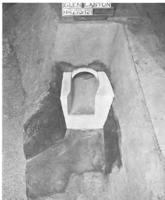
TRANSITION FLIP BUCKET WITH SIDE WALL DEFLECTOR Froude No. = 5.64 P-557-D-17051 & P-557-D-17052
