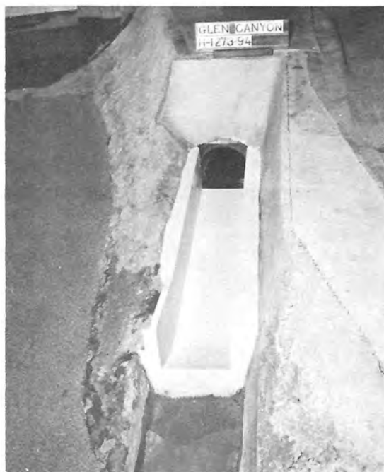
STANDARD FLAT BOTTOM FLIP BUCKET Flow at Froude No. = 7.89 P-557-D-17047 & P-557-D-17048
