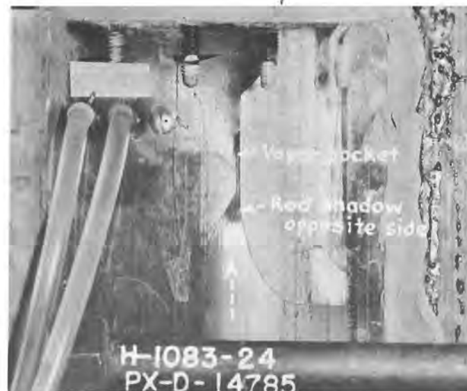
Fig. 18 Vapor Pocket in 1/4-inch long flow passage (width of flat face on gate seal ring) PX-D-14785
