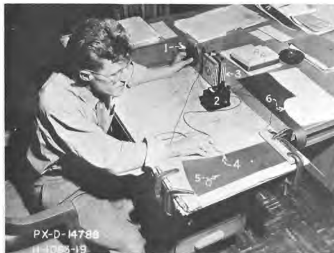
Fig. 15 Electric Analog Facility using graphite-coated paper to represent top seal flow passage. (1) Potentiometer (2) Galvanometer (3) Battery (4) Probe (5) Detail Seal Passage Cross Section 10 times prototype size (6) Boundary Curve 4 times prototype size. PX-14788
