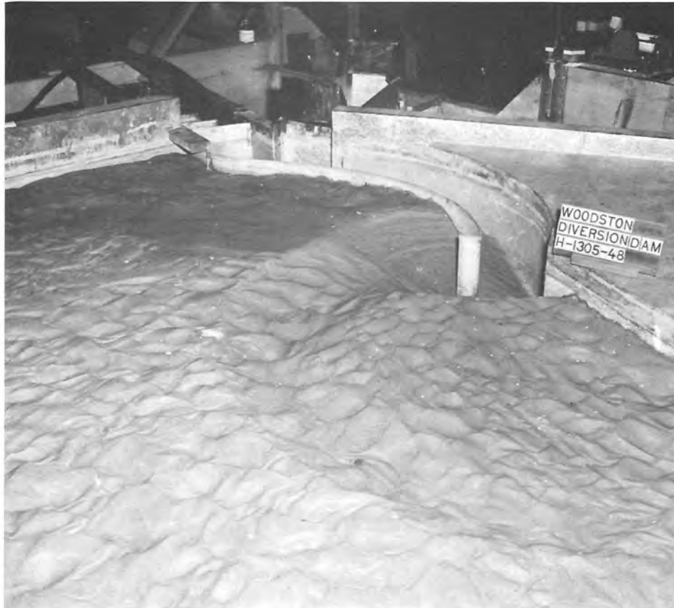
Movable bed hydraulic model study of Woodston Diversion Dam near Stockton, Kansas. The curved guide walls of the intake induced secondary spiral currents that caused the coarse bed material to move to the inside of the curve away from the canal intake and into the sluiceway. (H-1305-48)
