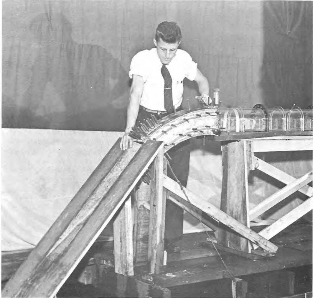
Model of typical river outlet used for concrete dams. A gate or valve controls the flow into the horseshoe tunnel and water is deflected downward along face of dam by vertical bend at end of conduit. (H-471-14)
