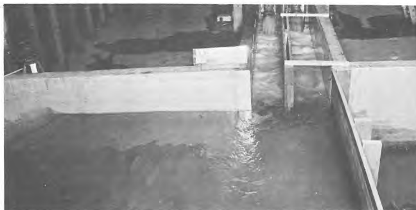
Figure 35. Flow Conditions Downstream of Hollow-Jet Valve Stilling Basin Utilizing Modified Hydraulic Jump.
