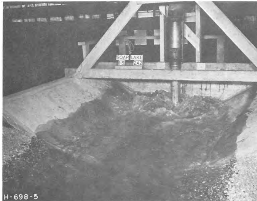
Figure 26. Soap Lake Siphon Blowoff--Preliminary 1:5 Scale Model Stilling Well--90 cfs.
