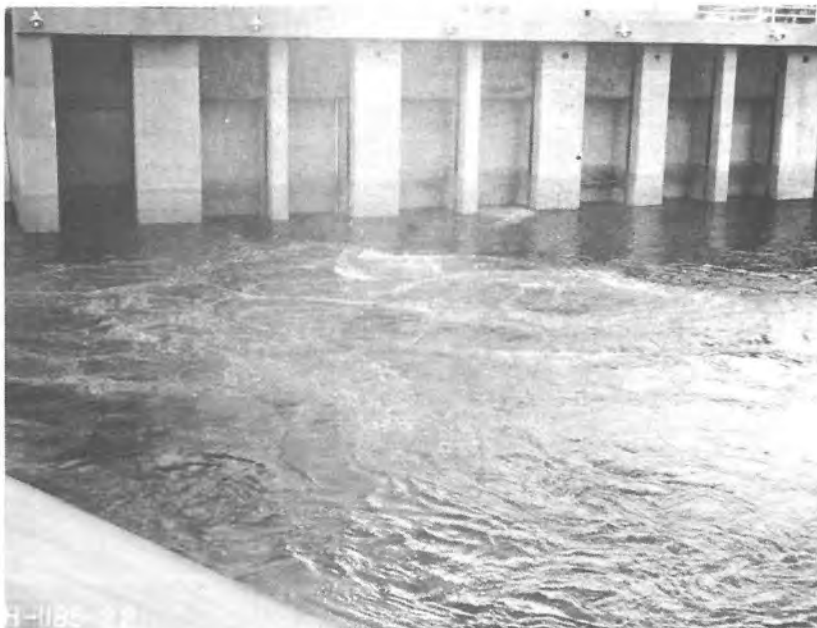
Figure 25. Flatiron Power and Pumping Plant--Flow in Tailrace Downstream of By-Pass Valve Stilling Basin--Air Injected Downstream of Baffle--Valve Fully Open.
