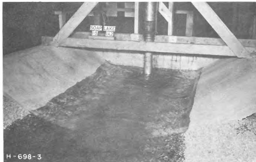
Figure 28. Soap Lake Siphon Blowoff--Final 1:5 Scale Model Stilling Well--90 cfs.
