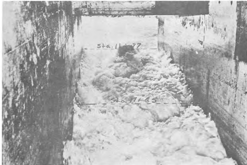
Figure 36. Flow Conditions in Boysen Dam Outlet Works Stilling Basin--730 cfs.
