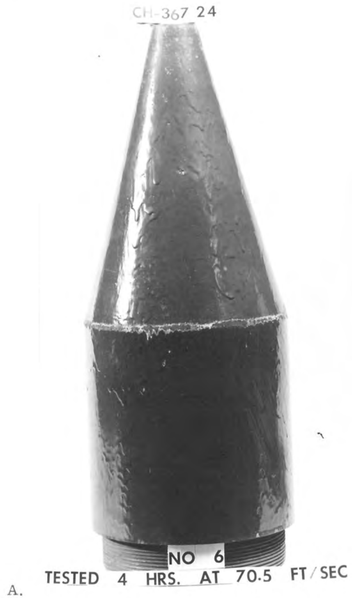
Tests of Protective Coatings SPECIMEN 6 AFTER 4 HRS At 70.5 FT/SEC.
