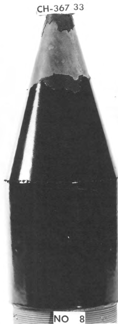
B. PITTING AT BASE AND TEAR AT TIP
