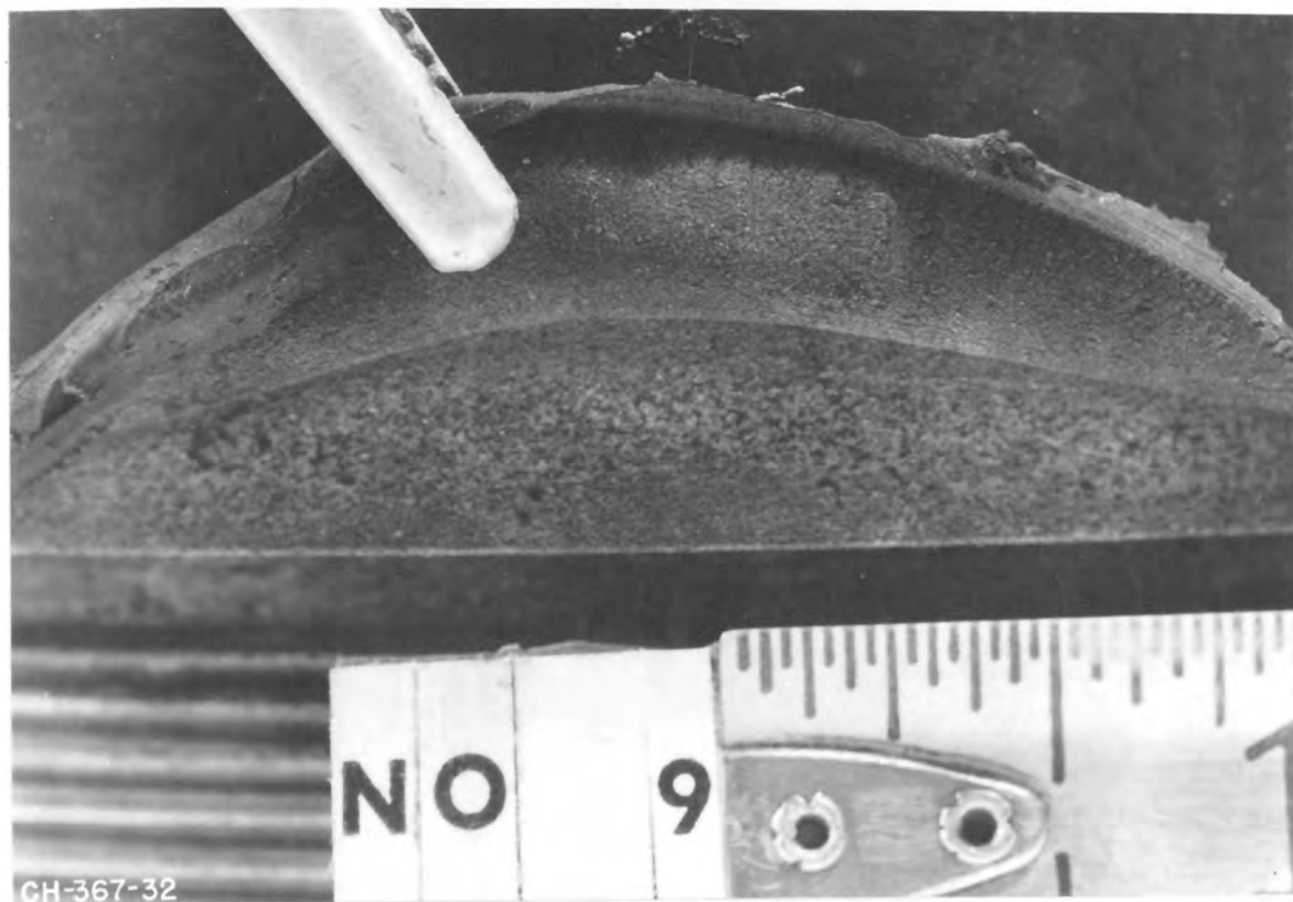
TEAR AT UPSTREAM EDGE OF COATING
