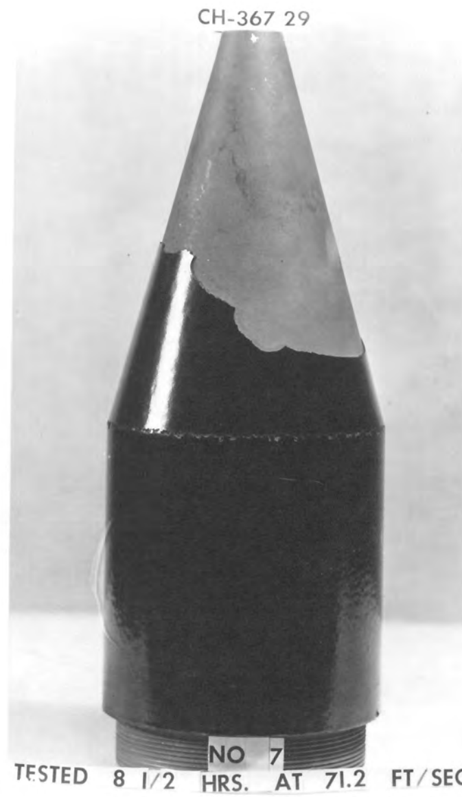
B. PITTING AT BASE - TEARING AT TIP RESULTING FROM LOOSENING BY CAVITATION
