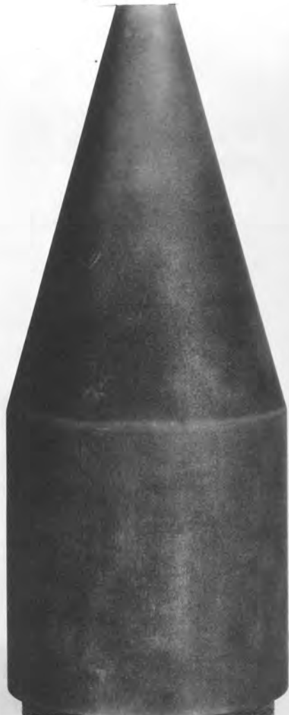
NO 3, UNCOATED SPECIMEN TESTED 11 1/4 HRS. AT 72.09 FT SEC A. METAL CONE SPECIMEN
