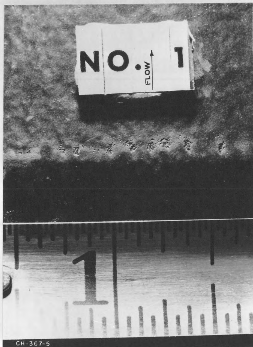
PITTED COATING AT CONE BASE
