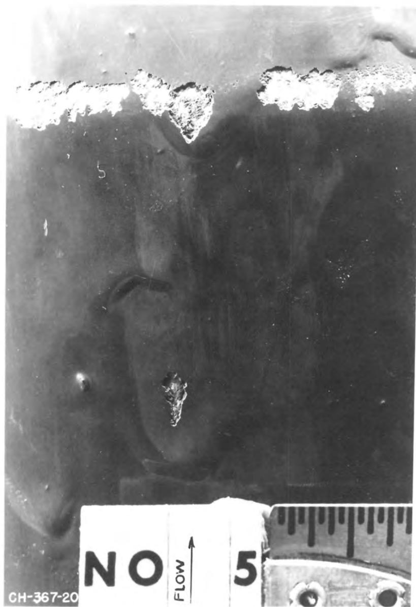
A. PITTING DOWNSTREAM OF COATING SAG IN STRAIGHT PART OF CONE SPECIMEN AND AT CONE BASE
