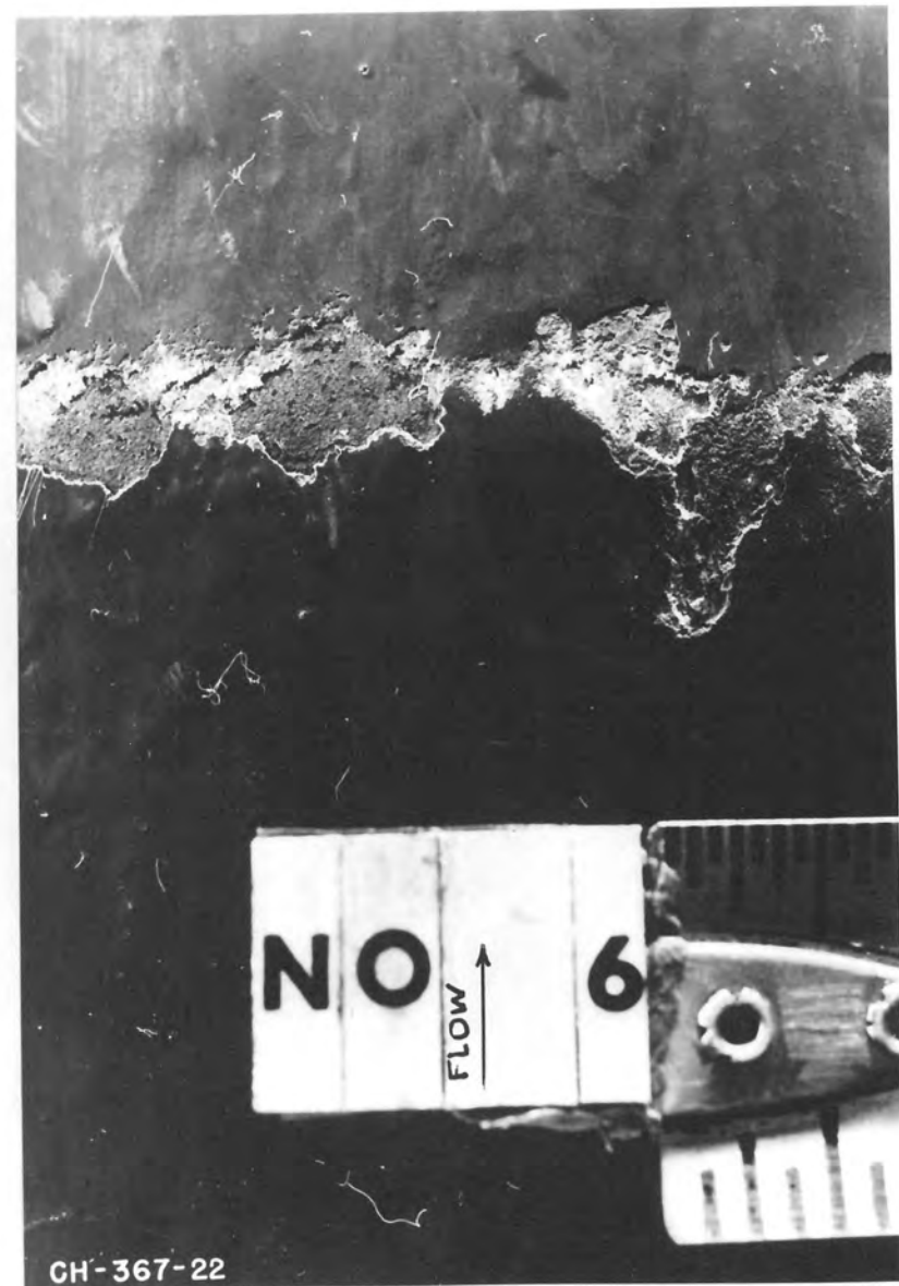
Tests of Protective Coatings SPECIMEN 6 AFTER 4 HRS At 70.5 FT/SEC.
