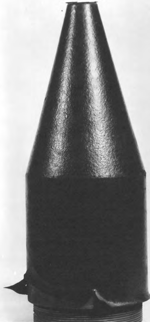
NO 2, FLAME SPRAYED THIOKOL TESTED 10 1/2 HRS. AT 71.2 FT/SEC
