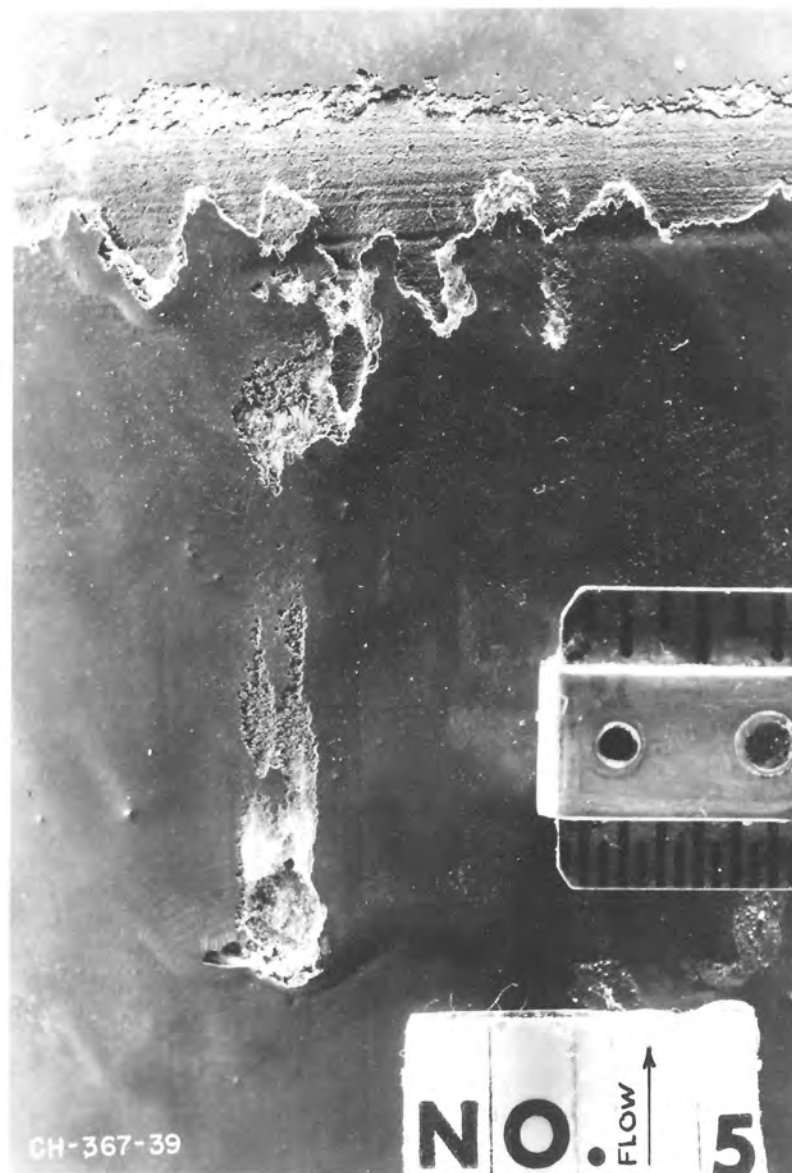
A. PITTING AT CONE BASE AND COATING SAG
