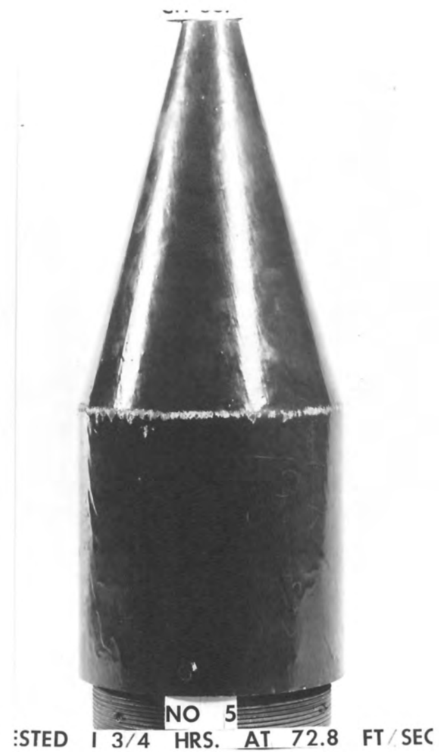
B. PITTING AT CONE BASE
