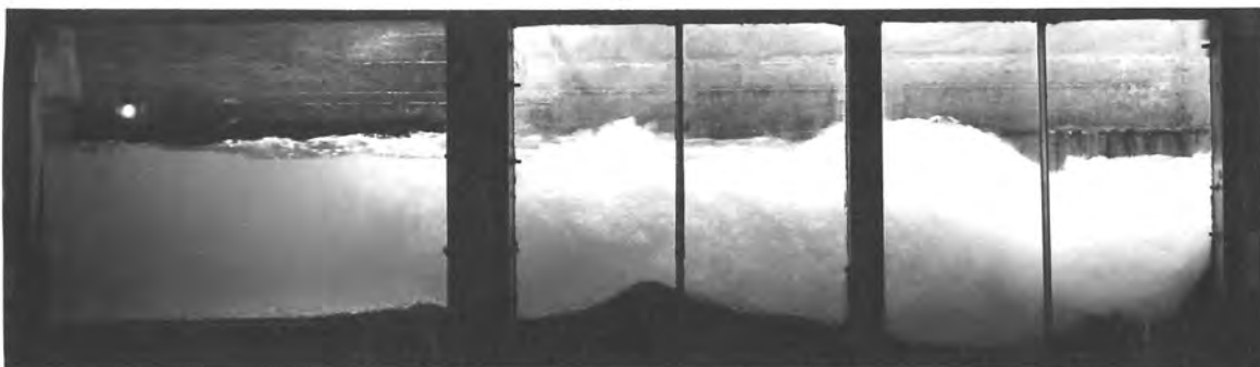
C. Tail-water depth exceeds the maximum limit but flow from the apron is lifted to the surface by a ground roller flow pattern which develops after the channel bed has been scoured sufficiently deep and the ground roller back fills the erosion hole
