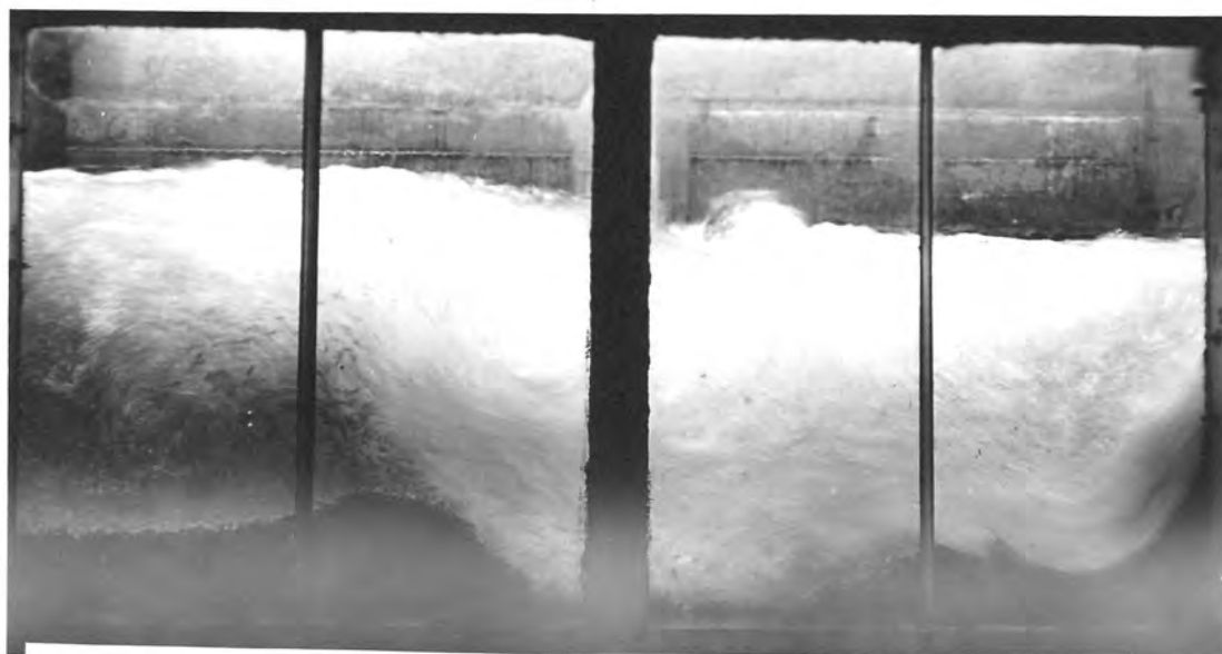
B. Tail-water depth (2.30 feet) exceeds the maximum limit
