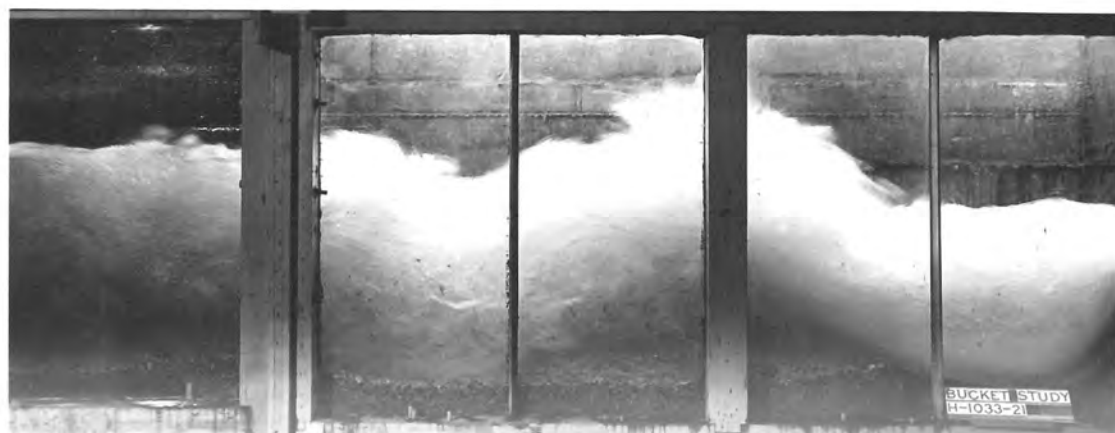
B. Angostura type bucket without slots and teeth Bucket radius 12 inches, discharge 6 cfs, tail-water depth 2.3 feet
