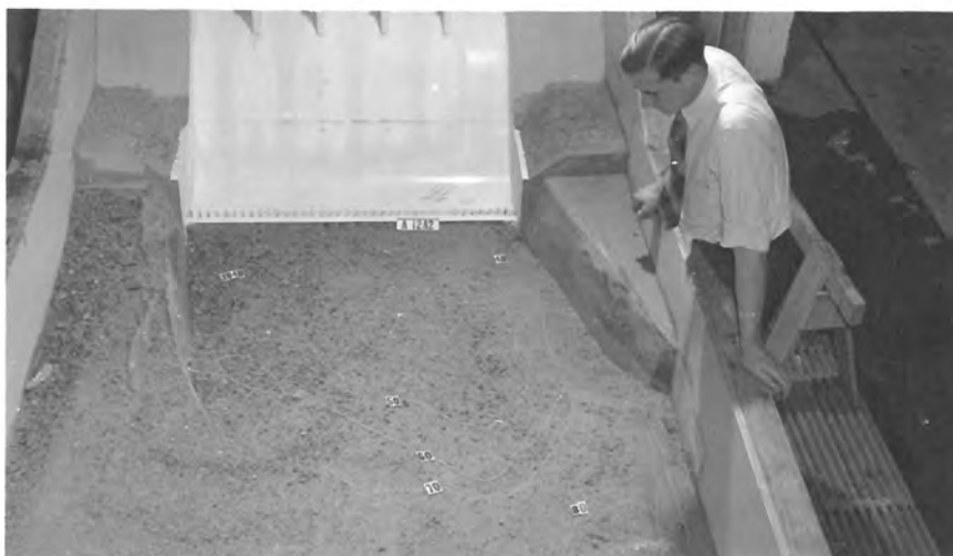
B - Erosion after flow of 277,000 second-feet for 20 minutes.
