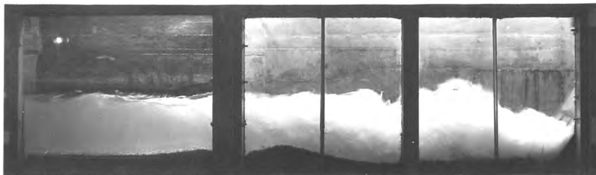
A. Normal operating conditions - tail-water depth between maximum and minimum limits being closer to the minimum
