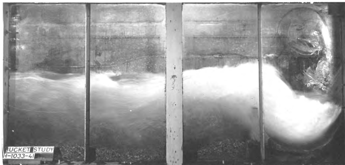
A. Discharge 6 cfs, tail-water depth 1.65 feet
