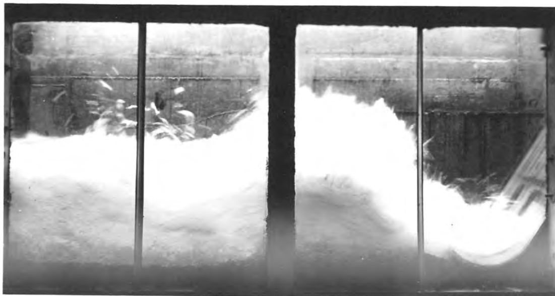
A. Tail-water depth (1.65 feet) is below the minimum limit
