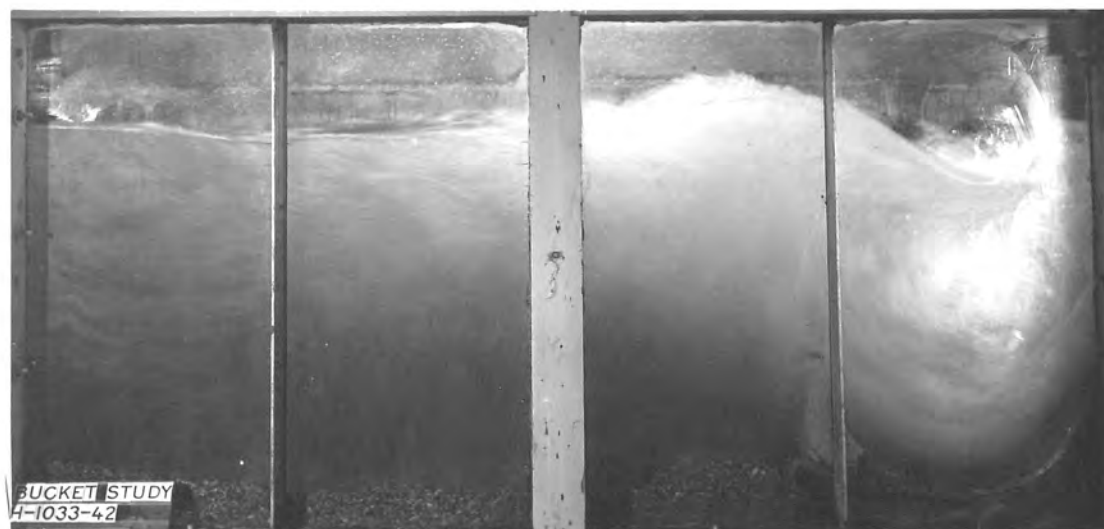
B. Discharge 6 cfs, tail-water depth 2.8 feet
