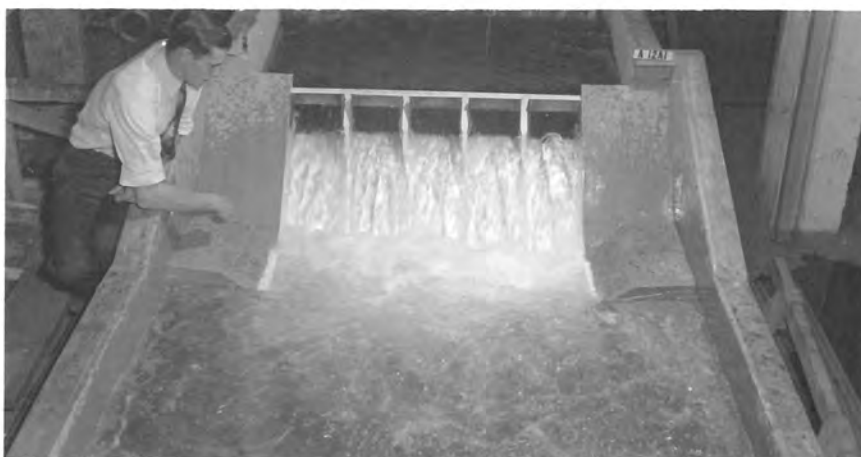
A - Flow of 277,000 second-feet over spillway.
