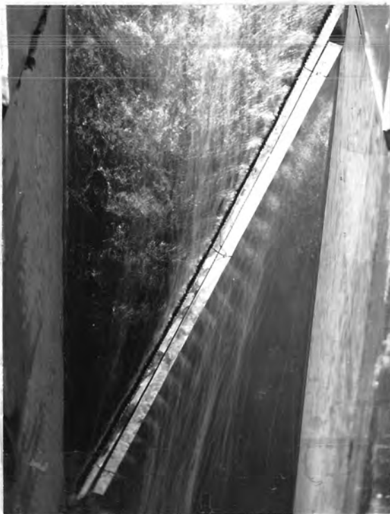
Figure 7--Flow lines through louvers--wide-spaced louvers separated from louvers by about 2 inches
