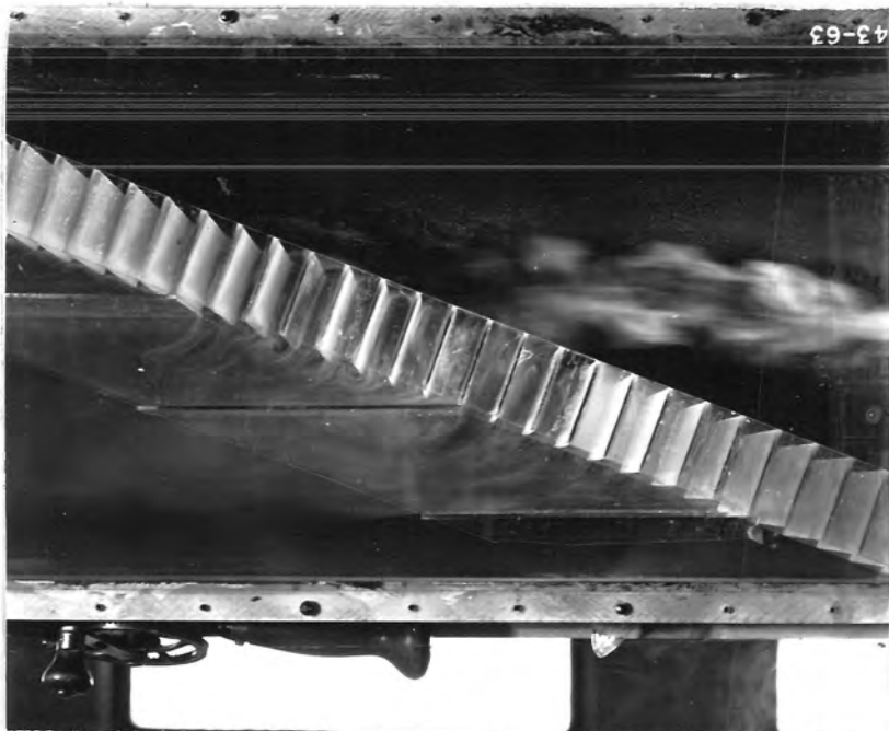
Figure 5-B--Flow lines through louvers--wide-spaced flow straighteners in place
