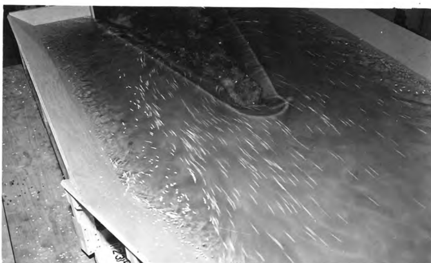
C. Large eddies occur where the canal widens for the weir Q = 16,000 cfs
