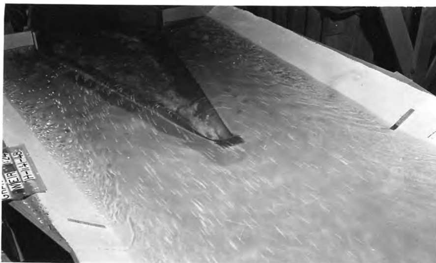
C. Smaller eddies occur with the warped transition walls than with the initial walls (see Figure 2C). Q = 16,000 cfs.
