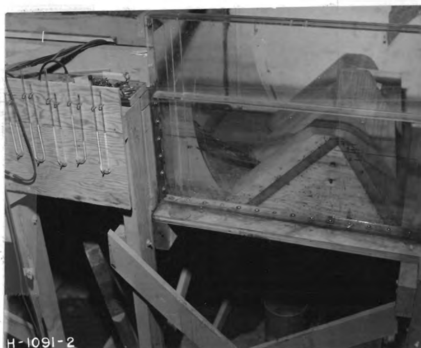
B Arch and buttress section model-scale 1:32
