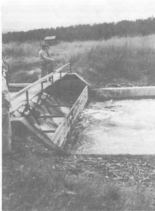
Figure 13. Model of Drop No. 4, Sunnyside Canal. Fully developed scour pattern after extended operation.
