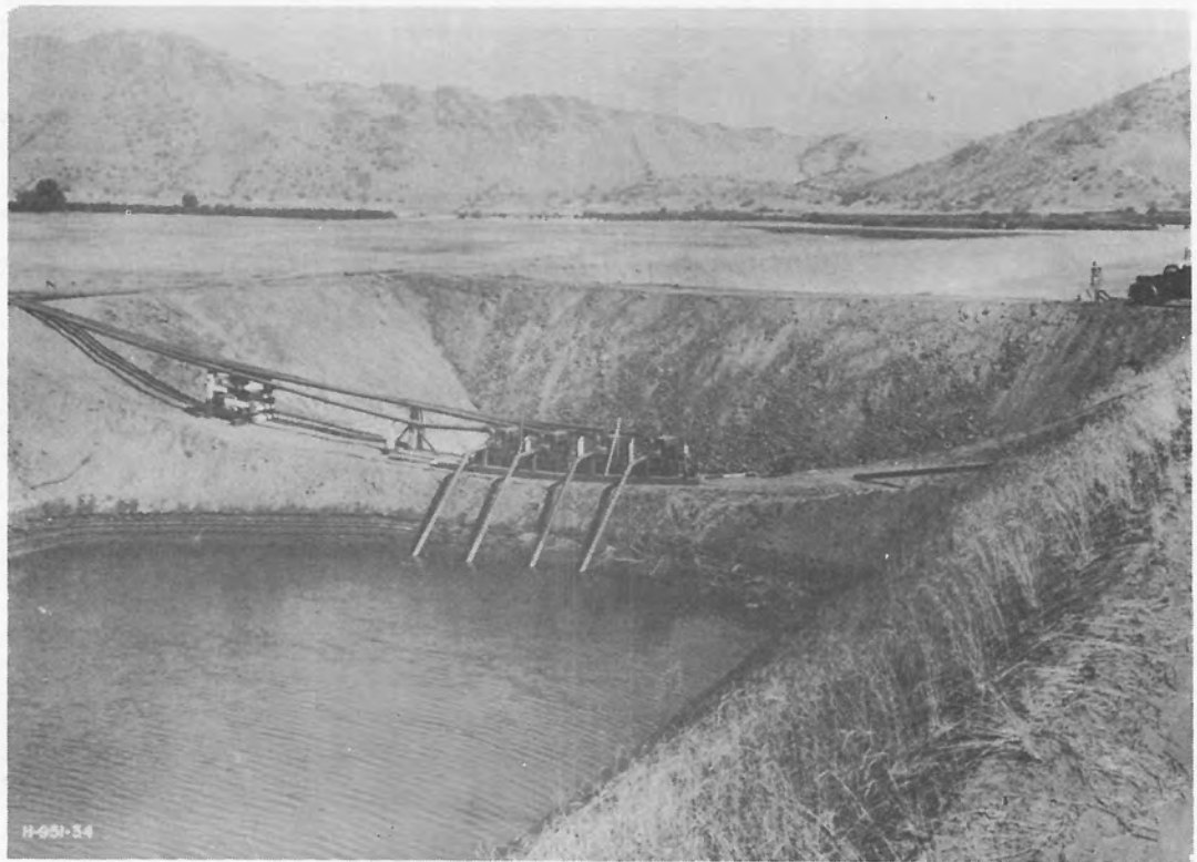
Figure 29. Determination of canal seepage losses by the ponding method.
