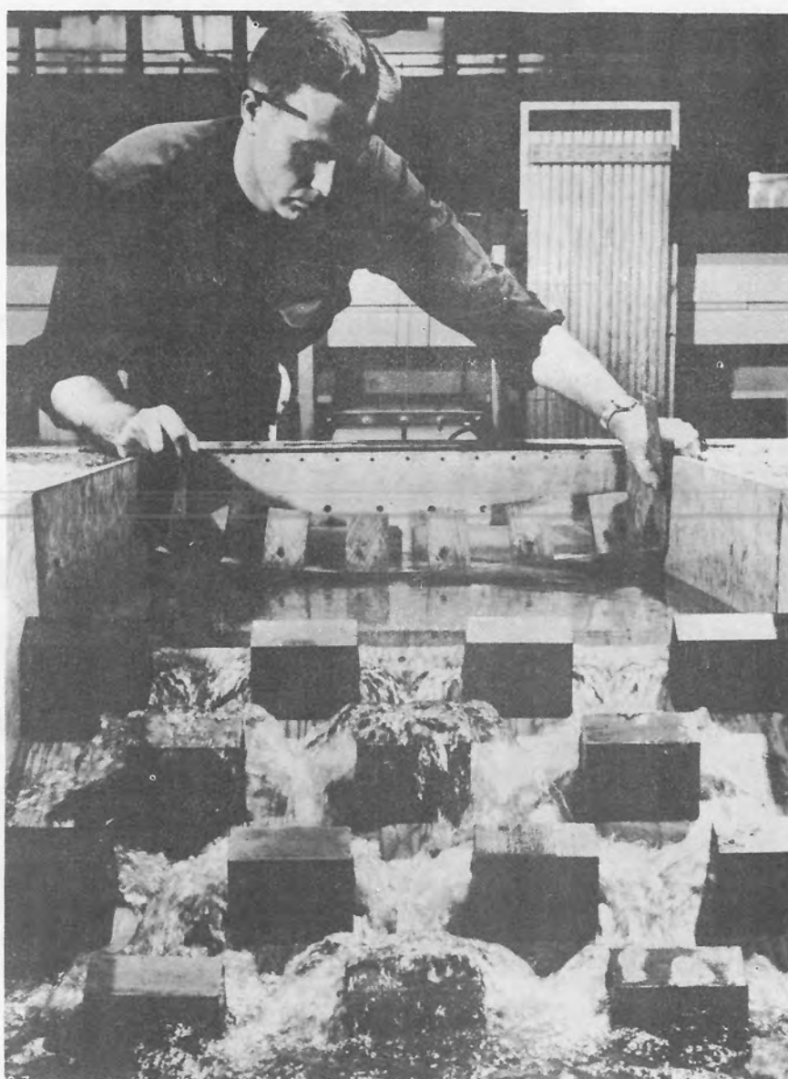
Figure 12. Typical overchute in which baffle piers are staggered.
