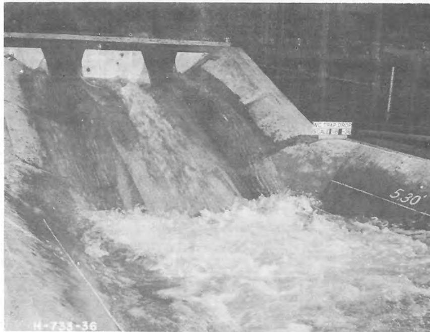
Figure 17. A 1:6 model of a trapezoidal concrete drop with two water stage-discharge control notches, Wyoming Canal.
