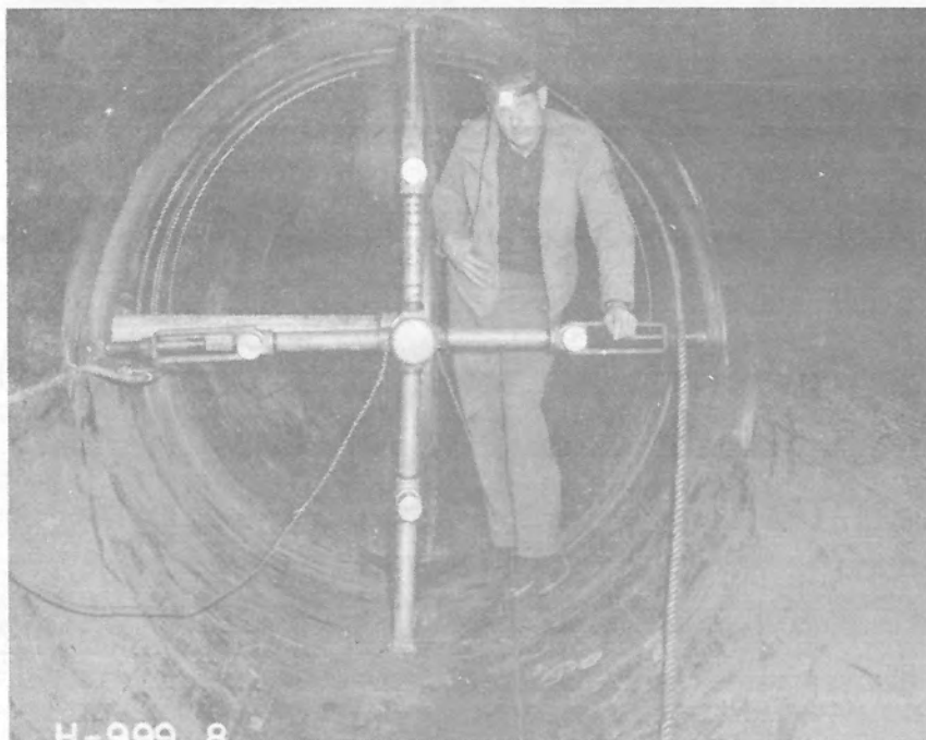
Figure 27. Injection station using pop valves in a 6-foot pump discharge line.
