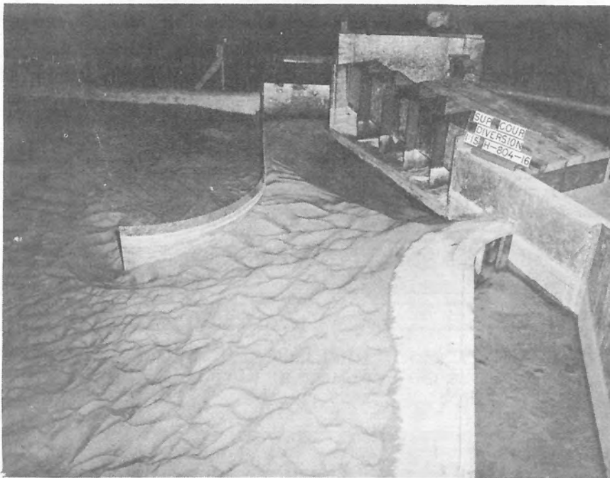
Figure 24. 1:15 model of Superior-Courtland Diversion Dam--Superior Canal headworks. (Nebraska).
