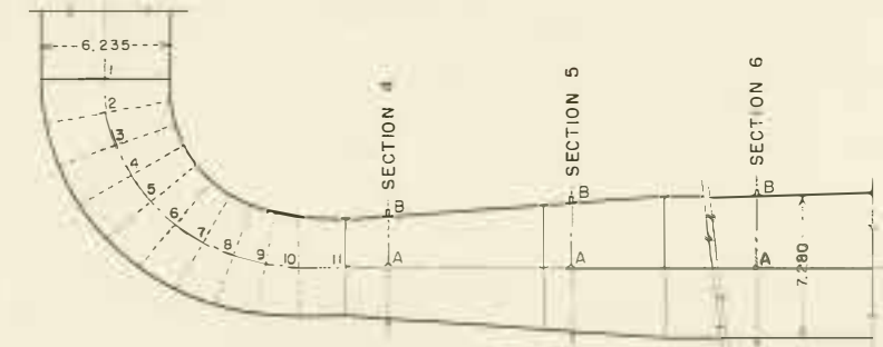
BEND No. 7 SINGLE CONICAL DISCHARGE = 2.988 C.F.S.
