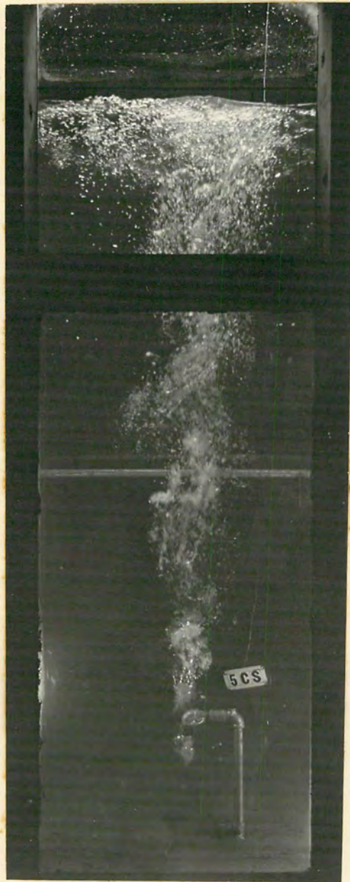
Figure 3 - Typical vertical discharge flow pattern at 3 pounds per square inch differential pressure (orifice C).
