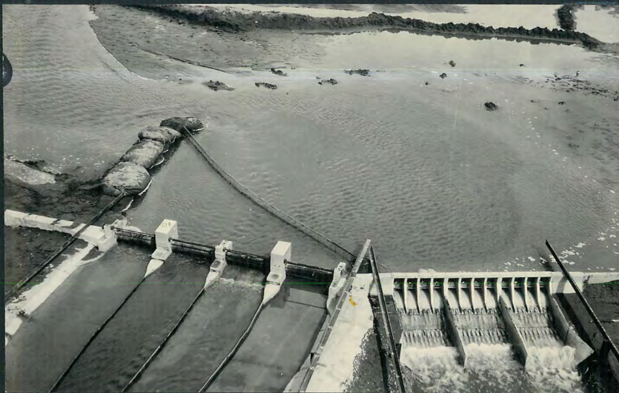
Layout No. 22 - Flow conditions with river from right Intake Q = 10,000 Sluiceway Q = 14,000
