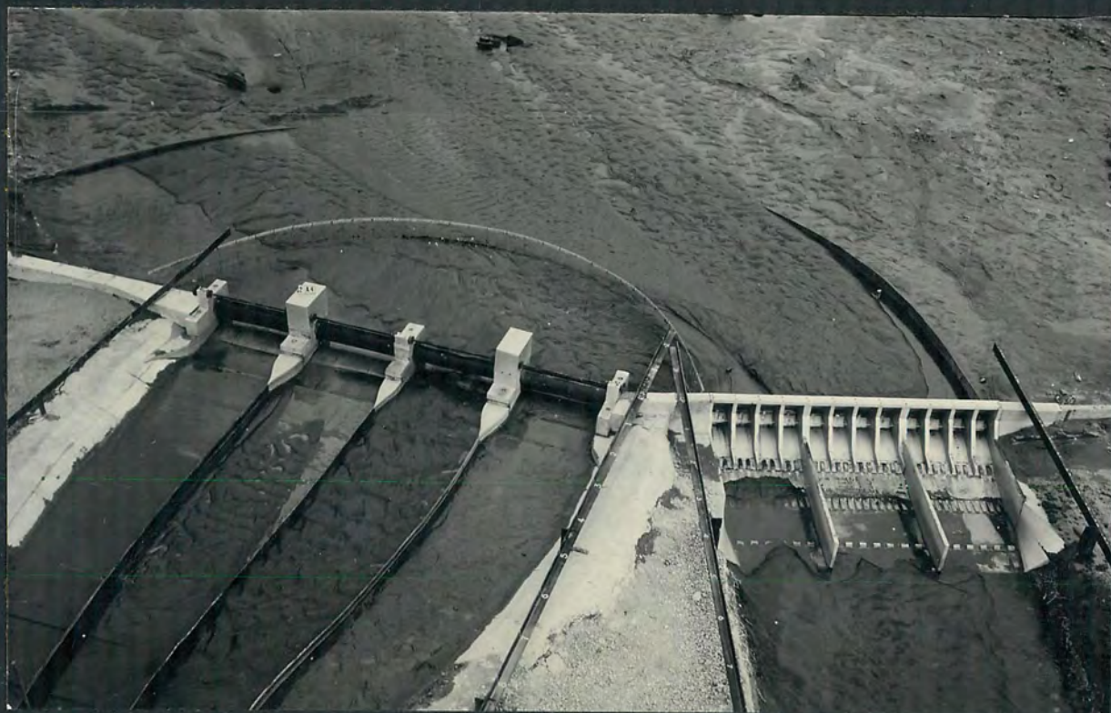
Layout No. 2 - Trashrack in position A - Silt deposit after 6-hour run with river from right - Intake Q - 10,000 Sluiceway Q - 14,000
