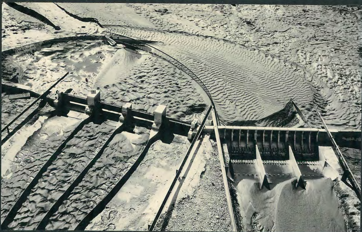
Layout No. 1 - Trashrack in position B - Silt deposit after 6-hour run with river from right Intake Q = 10,000 Sluiceway Q = 14,000
