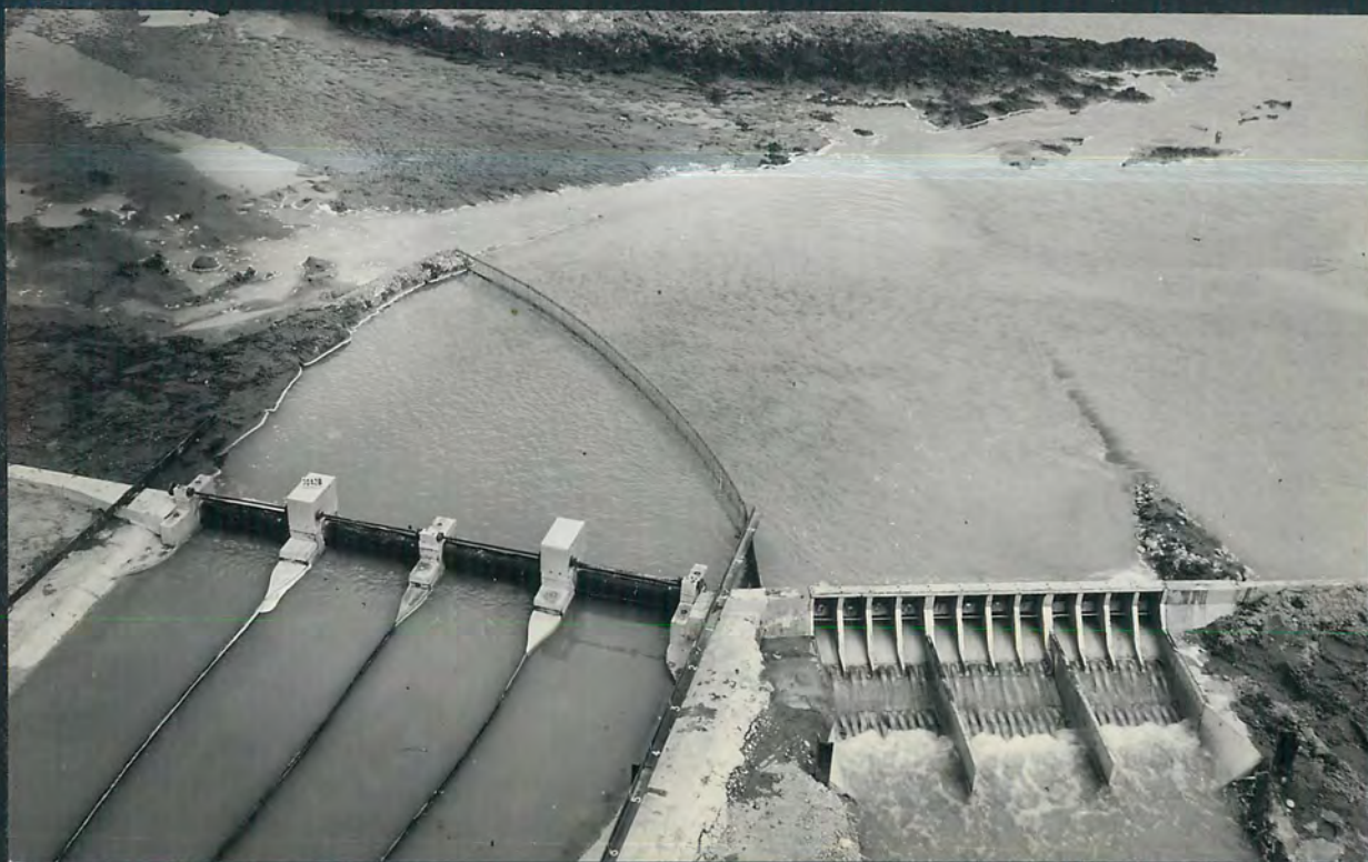
Layout No. 30 - Flow conditions with river from left Intake Q = 10,000 Sluiceway Q = 14,000
