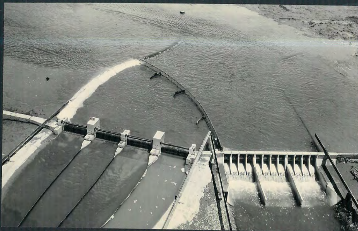
Layout No. 6 - Flow conditions with river from right - Intake Q = 10,000 Sluiceway Q = 1,000
