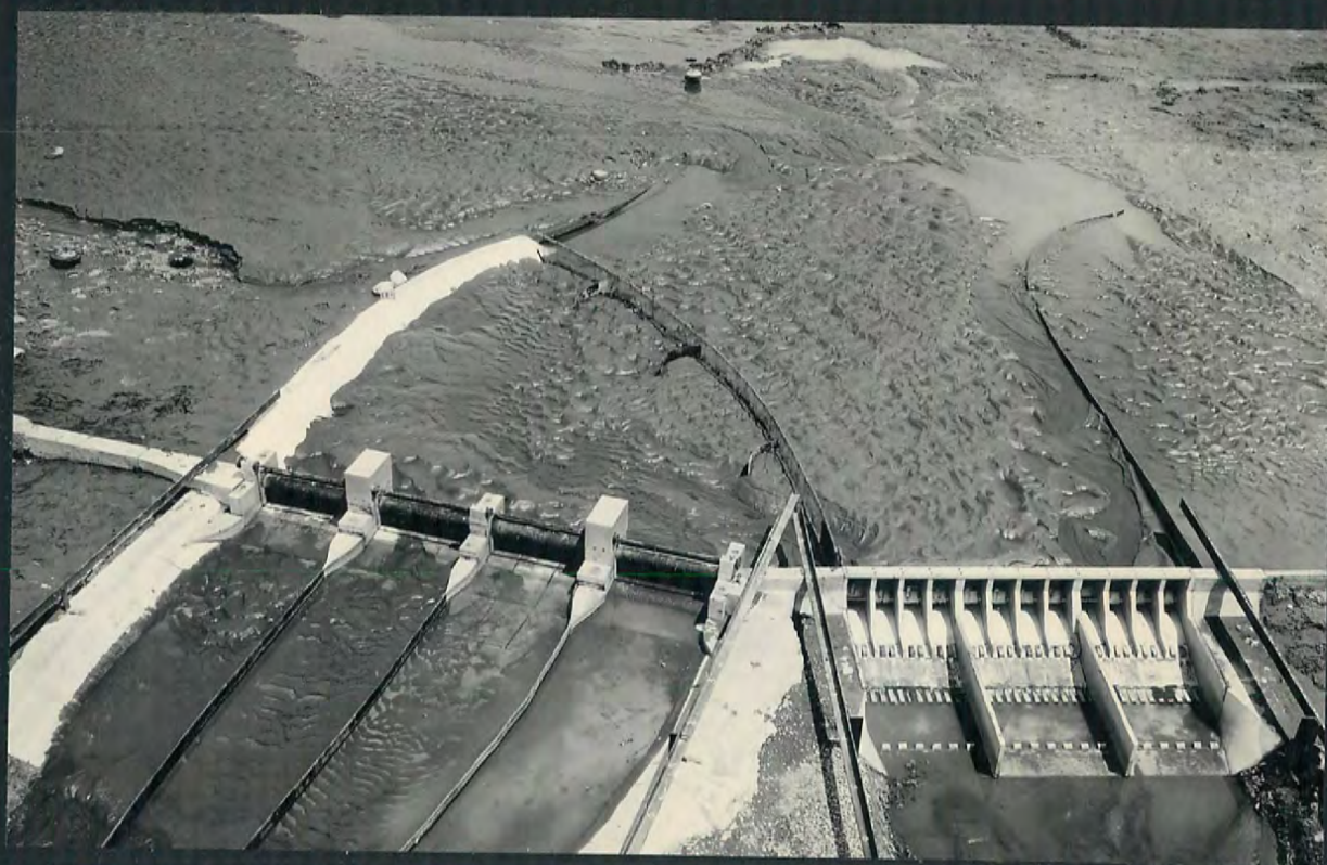
Layout No. 7 - Silt deposit after 1\frac{1}{2} -hour run with river from right Intake Q = 10,000 Sluiceway Q = 14,000
