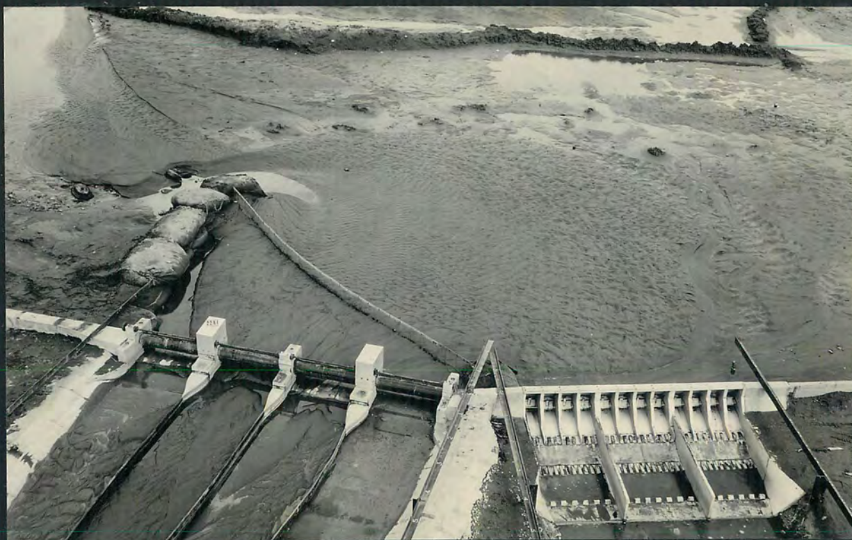
Layout No. 22 - Silt deposit after 3-hour run with river from right Intake Q = 10,000 Sluiceway Q = 14,000
