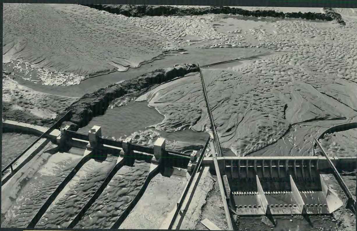
Layout No. 19 - Silt deposit after 6-hour run with river from right Intake Q - 10,000 Sluiceway Q - 14,000
