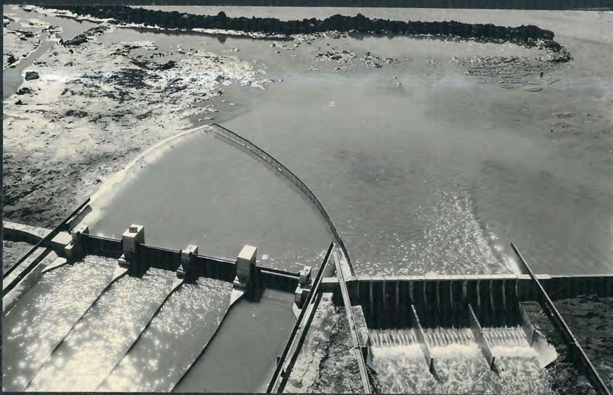
Layout No. 12 - Flow conditions with river from left Intake Q = 10,000 Sluiceway Q = 14,000
