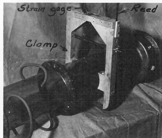
View of vibration clamp showing reed and De Forest strain gage.
