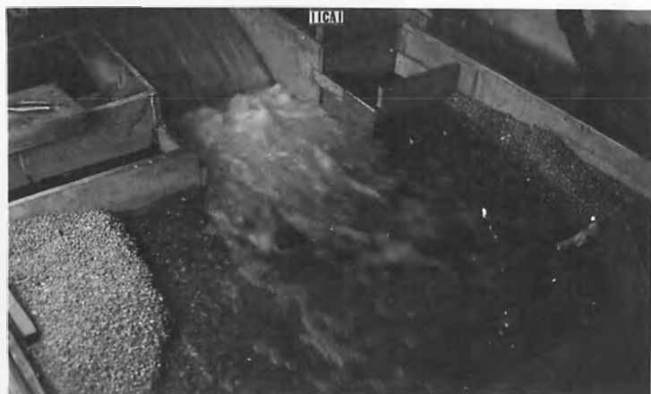
D. Final Design - Discharge 34,100 c.f.s.
