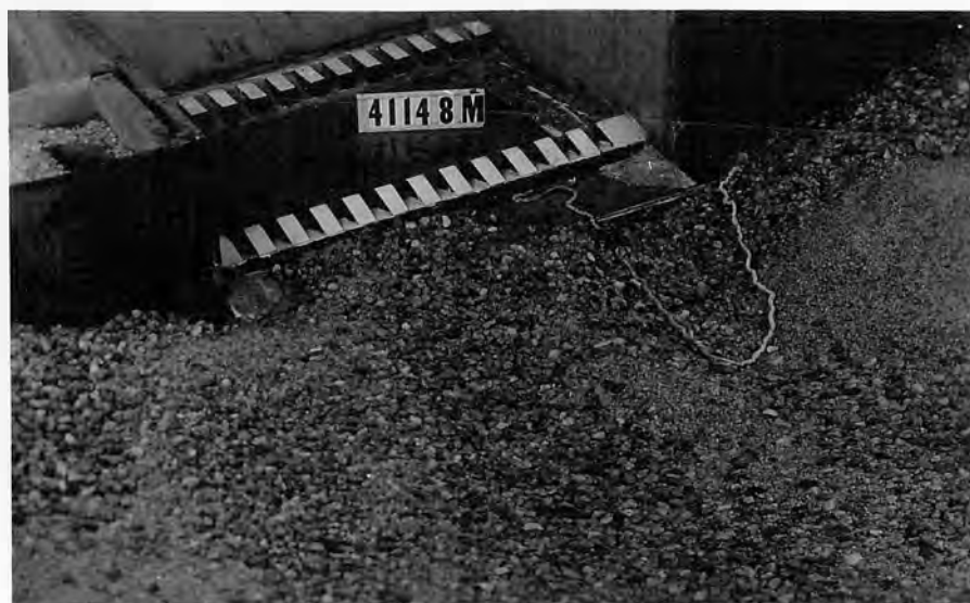
SCoured BED - 33,000 C.F.S. 2 HRS. @ 4114 T.W., \frac{1}{2} HR. @ 4118 T.W.
