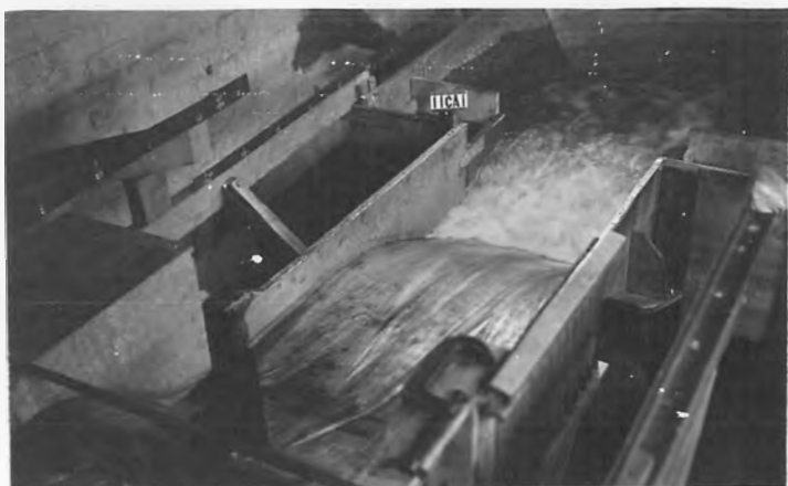
A. Final Design - Discharge 34,100 c.f.s.
