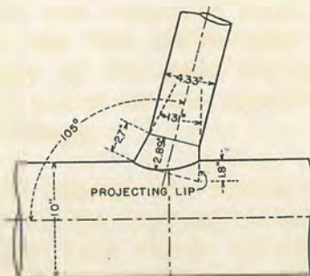
B-SKETCH OF LIP IN MAIN PENSTOCK AS USED IN A AND B-FIGURE 4
