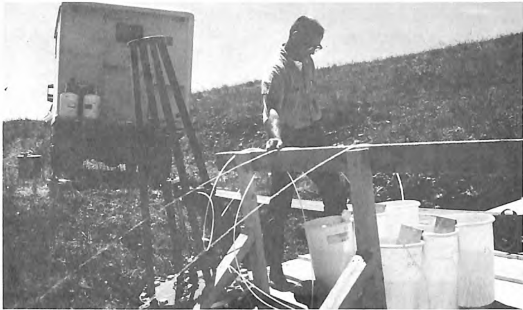
Mobile Nuclear Laboratory at Sampling Point 105 Diameters from Injection—Sample Containers and Timer on Platform. Photo P245-D-63691NA
