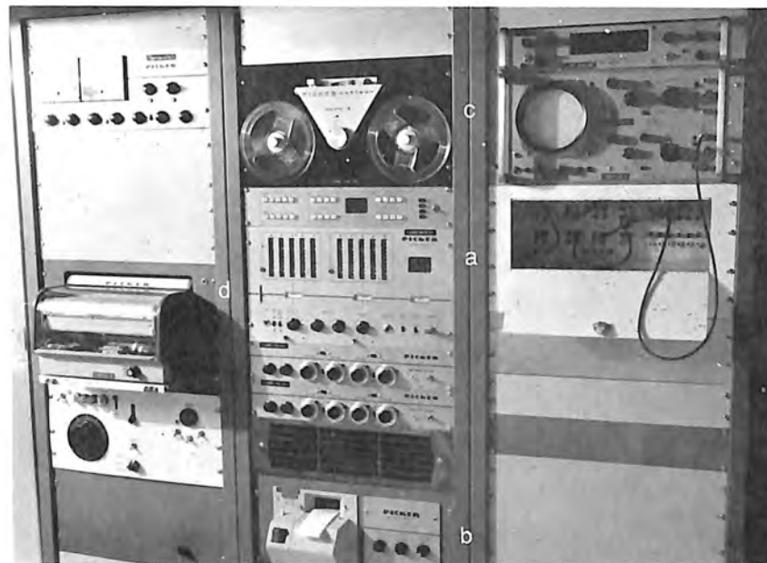
Radiation Counting and Recording System Installed in Mobile Laboratory (a) Scaler (b) Printer (c) Magnetic Tape (d) Analog Recorder. Photo PX-D-64665
