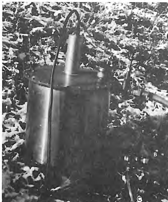
Sample Tank Containing Detector and Connected to Penstock Sampling System—Tube (a) To Drain, Tube (b) From Penstock, Tube (c) For Integrated and Diluted Samples. Photo P245-D-63704NA
