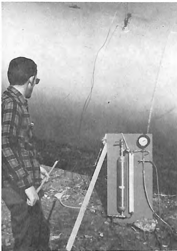
Tracer Injection System for Dilution Method—Tube at Bottom of Cylinder was Connected to the Four-outlet Manifold. Photo P245-D-63702NA
