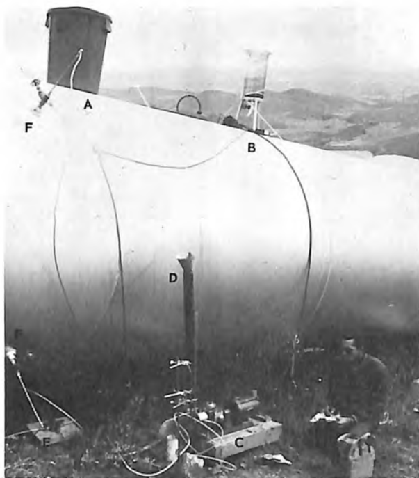
Fluorescent Dye Injection System (a) Water (b) Dye Mixing Tank (c) Diaphragm Chemical Feed Pump (d) Buret for Injection Rate Measurement (e) Injection Manifold, and (f) Two of Four Injection Tubes. Photo P245-D-63696NA
