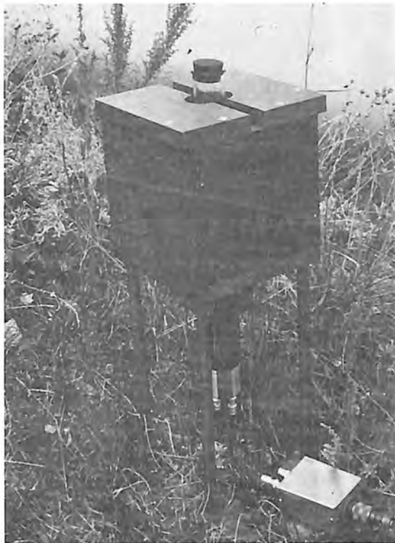
Radiation Counting Flask in Shield-Disc Scintillation Counter and Photomultiplier Mounted Below Flask in Shield Opening. Photo P245-D-63693NA
