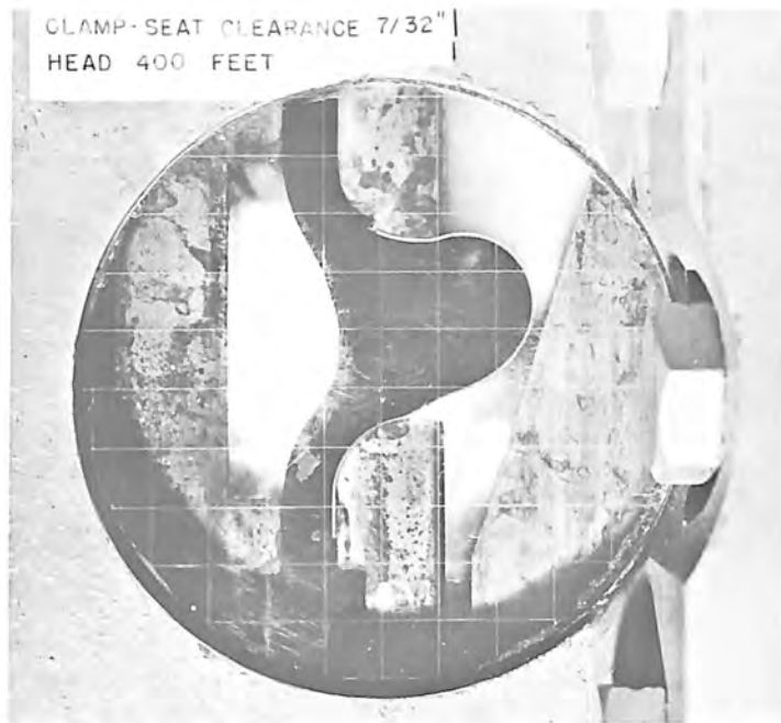
A. Seal bulb extended during closing cycle. Photo PX-D-60637
