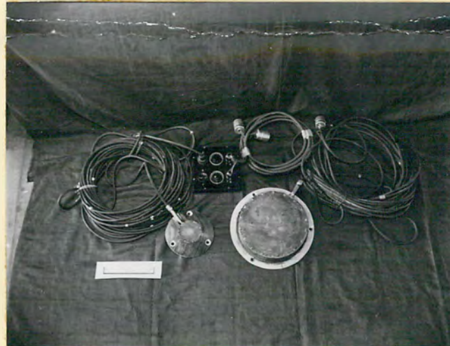
PRESSURE CELLS USED TO OBTAIN FREQUENCY AND AMPLITUDE OF FLUTTER-CARBON FILE PRESSURE CELL (LEFT) - MOVING - COIL PRESSURE CELL (RIGHT) - CONTROL BOX (CENTER)
