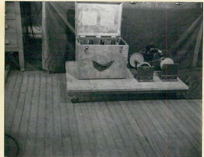
VIEWS OF SHAKING TABLE USED TO CALIBRATE ACCELEROMETER UNITS
