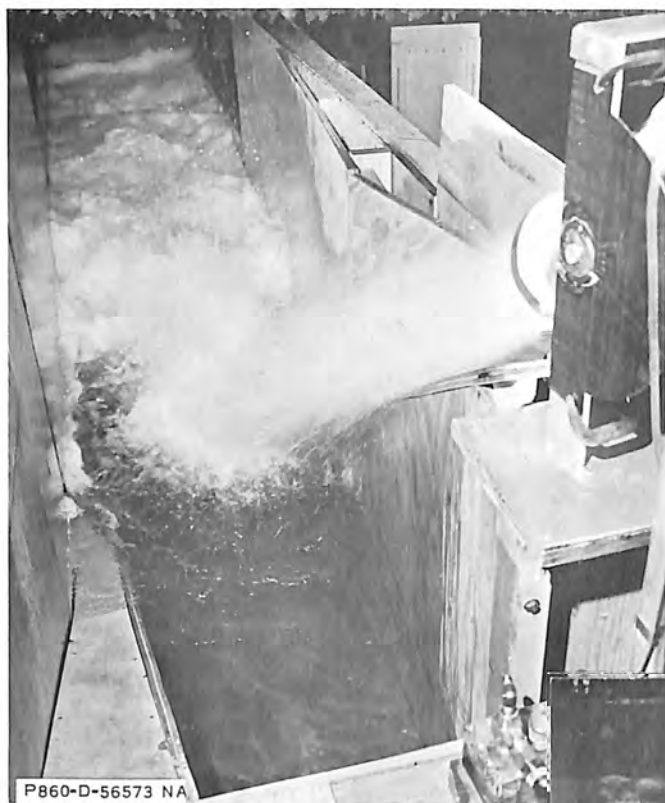
Above - Discharge 36 cfs 59 feet of head
