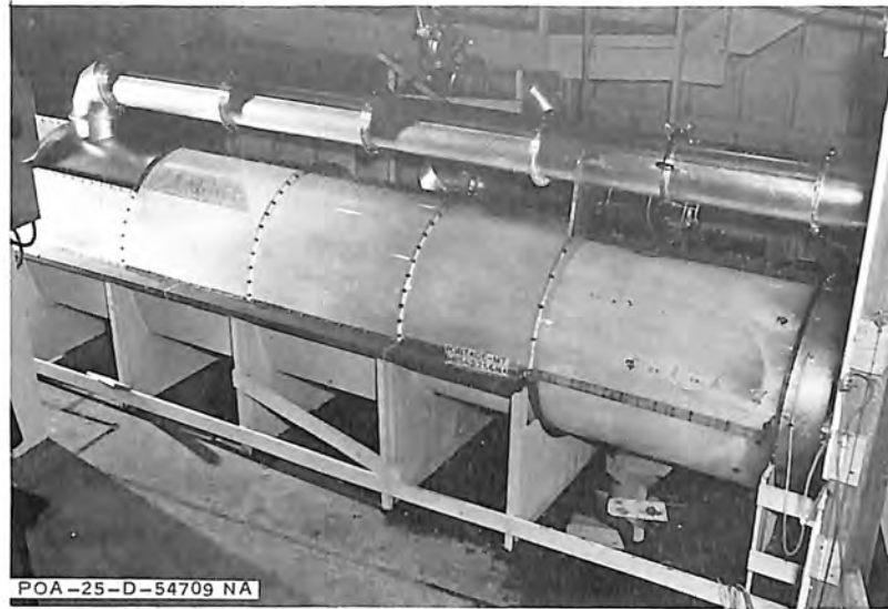
A. Jet trajectory from barrel liner extends beyond entrance to overhead air tunnel.
