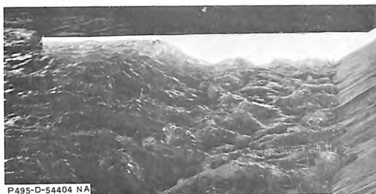
Preliminary baffle piers - Discharge 264,500 cfs tailwater El. 1431 gates fully open
