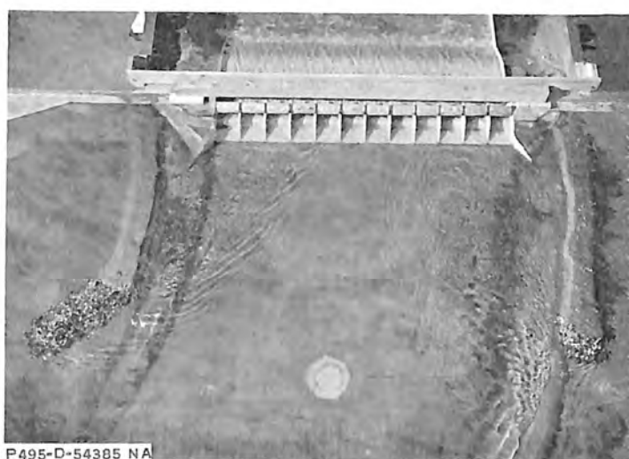
The upstream end of the left dike placed 30° away from the approach channel. Discharge 264,500 cfs; fully opened gates; reservoir water surface El. 1492.2
