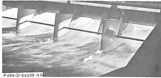
A. Flow through bays and clearance of pilaster modeled in the left end bay. Discharge 264,500 cfs; reservoir water surface El. 1492.2
