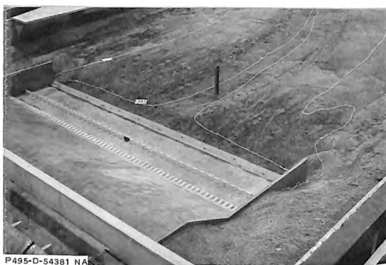
B. Erosion after operation for 2 hours (prototype) at 264,500 cfs
