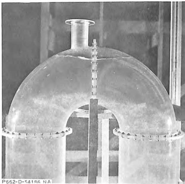
C. No air entrained - flow tranquil with bend partially full.
