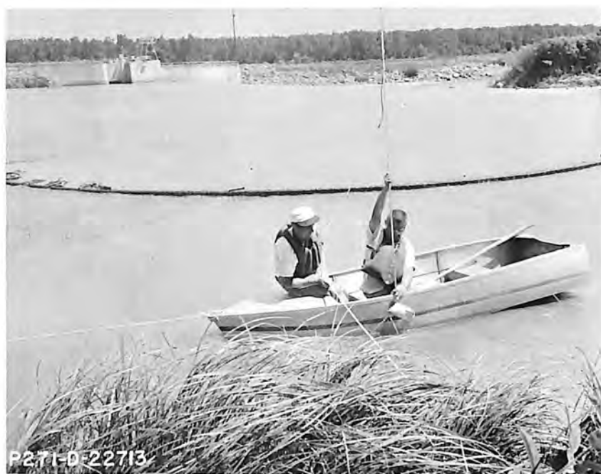
A. Obtaining suspended sediment sample using DH-48 sampler from a boat.
