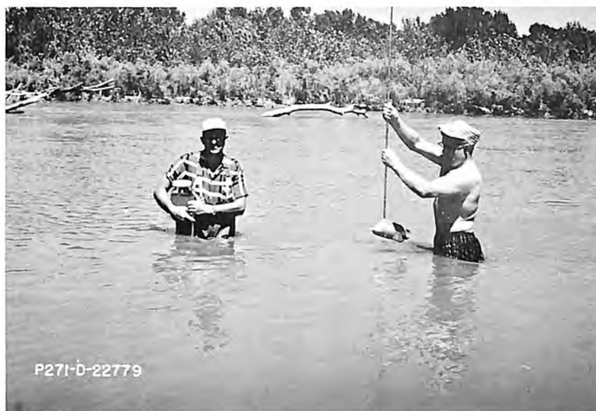
A. Sampling with DH-48 sediment sampler in Republican River upstream from Superior-Courtland Diversion Dam.
