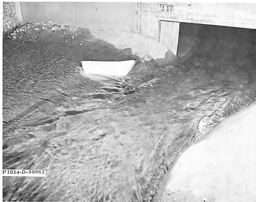
A. Straight guide wall to reduce scour.
