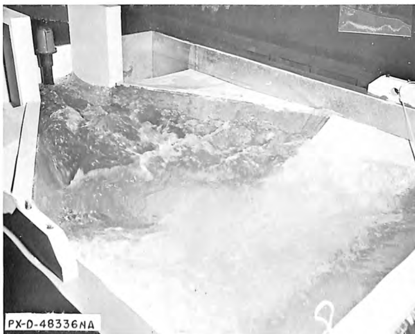
B. Farm turnout model with water at design depth, Discharge = 5.0 cubic feet per second.
