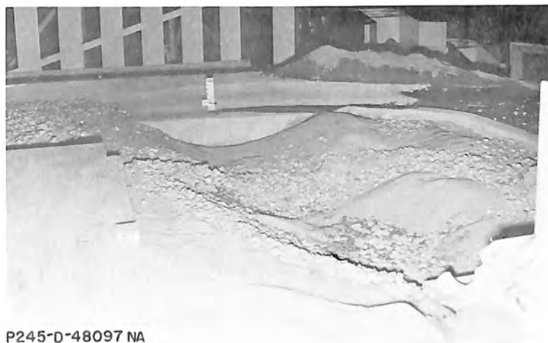
B. Erosion after 12,000 cfs
