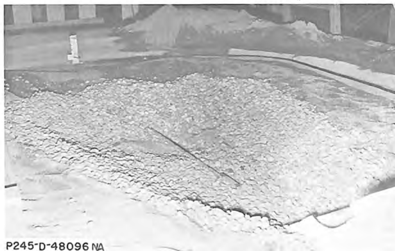
A. Erosion after 3,000 cfs
