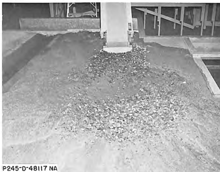
B. Erosion caused by 1,200 cfs discharge
