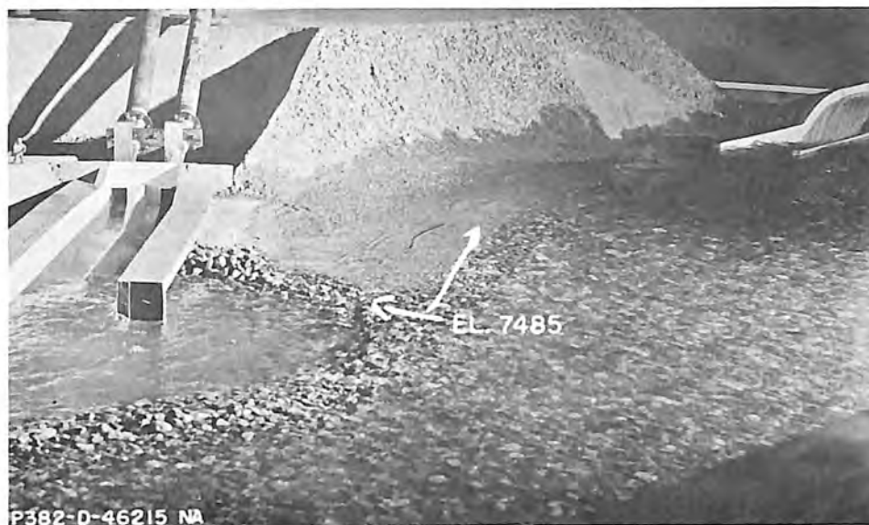
A. Submergence and washing of unprotected area downstream of bypass stilling basin.
