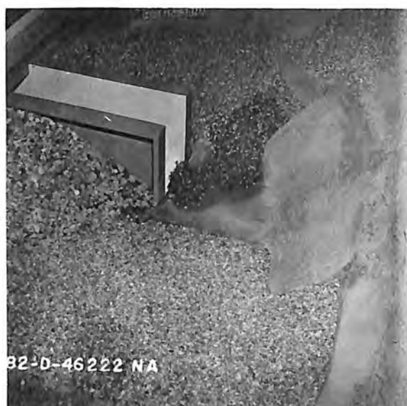
B. Scour after 20 prototype hours' operation at 5540 cfs.
