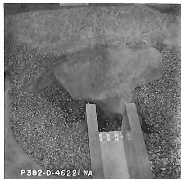
B. Scour after 20 prototype hours' operation at 5540 cfs.
