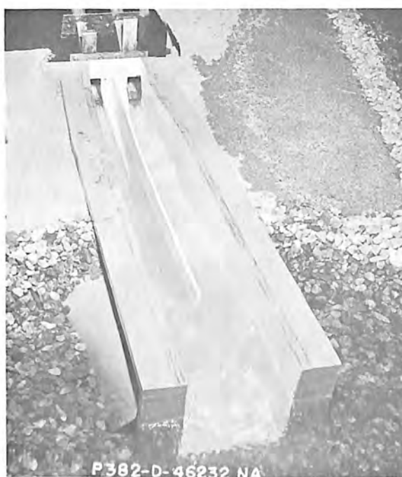
B. Left gate only operating Q = 975 cfs; T. W. El. = 7480.5
