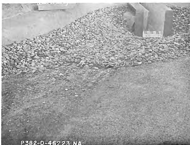
A. Erosion in unprotected channel downstream of outlet works after 26 prototype hours' operation at 1950 cfs.
