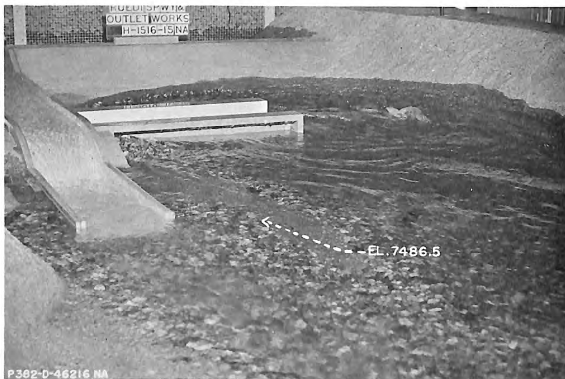
B. Wave action across submerged area on left of bypass stilling basin.
