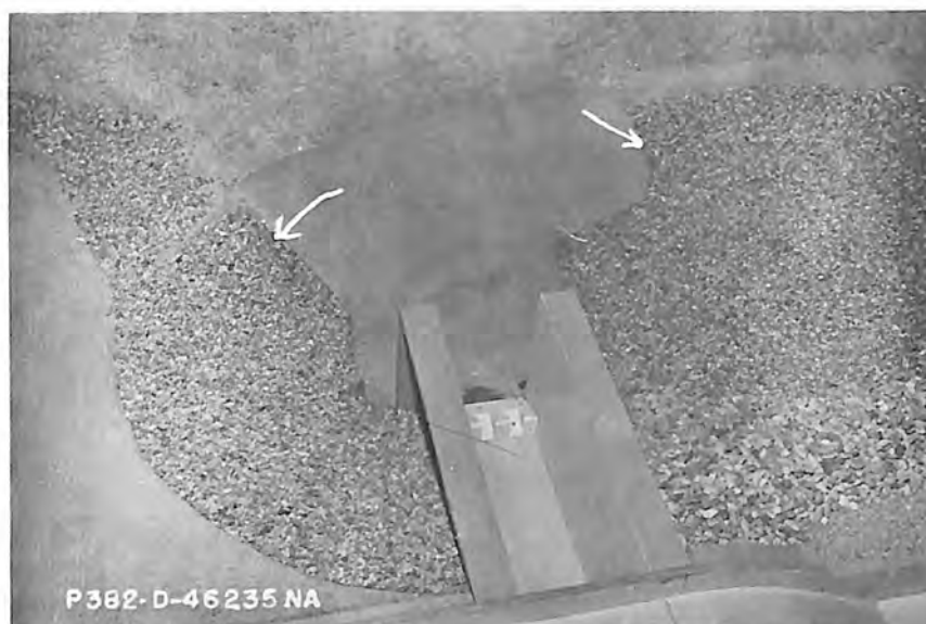
A. Smaller riprap (10- to 15-inch prototype) before test. Arrows point to assumed limits of exposed rock, at 1.5:1 slope.
