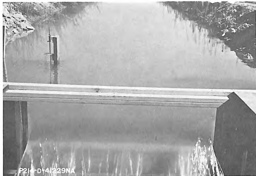
A. Weir performance for nappe vented with discharge of 24.9 cfs.
