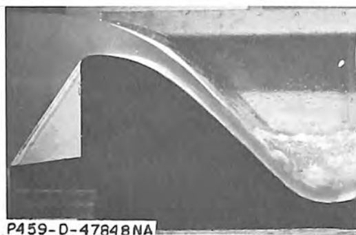
A. Maximum discharge 3,100 cfs per bay (15,500 cfs total). Reservoir elevation 3189.5, tailwater elevation 3165.5.
