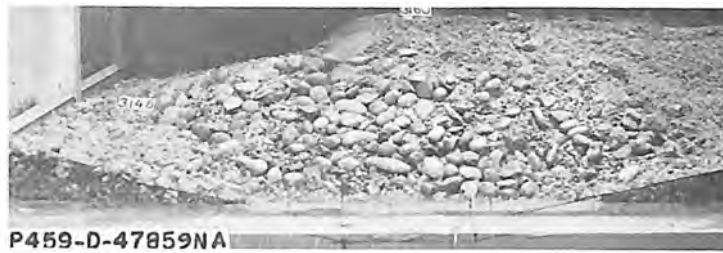
A. Riverbed downstream from the basin before erosion test.
