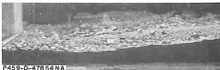
C. The riverbed after a 2-hour (prototype) erosion test at maximum discharge. Seven dentates per bay, preliminary end sill.
