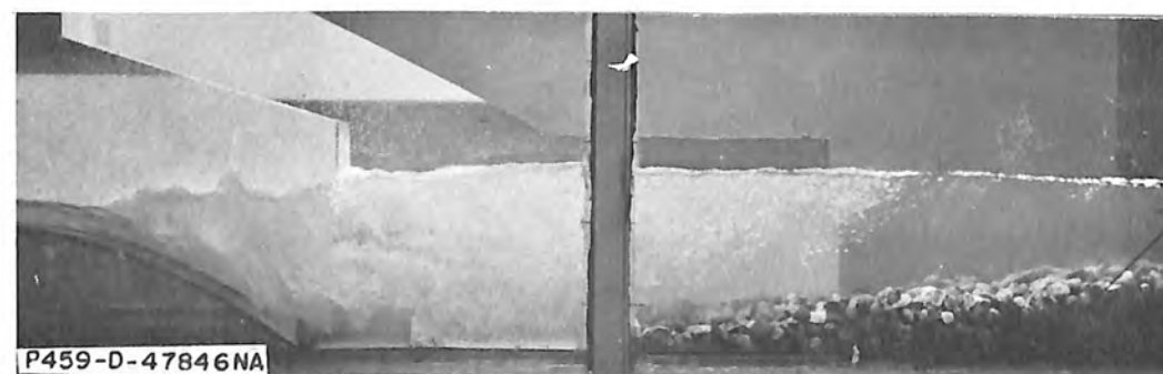
B. Reservoir elevation 3189.5, tailwater elevation 3161.5. Gates 63 percent open.
