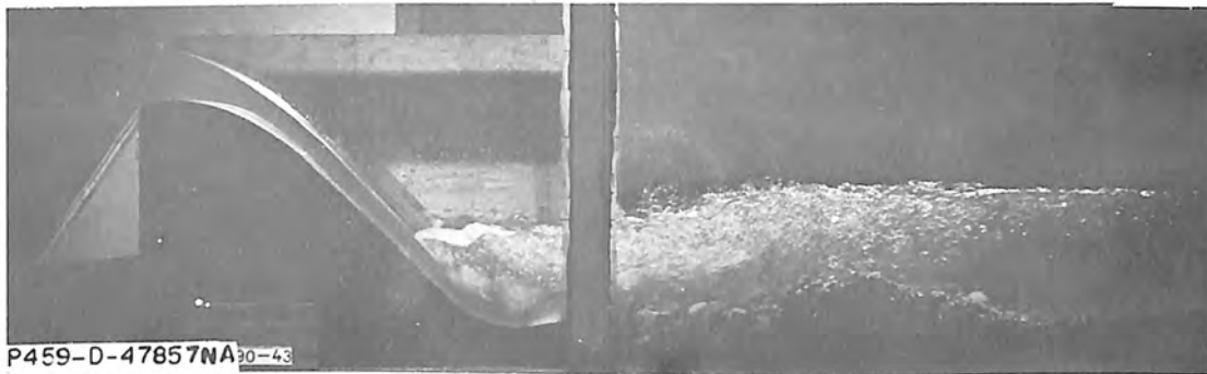
A. Basin with 12 dentates per bay with 12-inch spaces between dentates and the initial ( 18^\circ rise) end sill.
