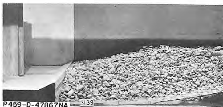
B. Result of the 2-hour erosion test with maximum Q tailwater elevation 3165.5.
