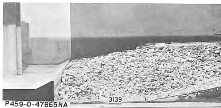
A. Arrangement of riverbed and riprap prior to testing.
