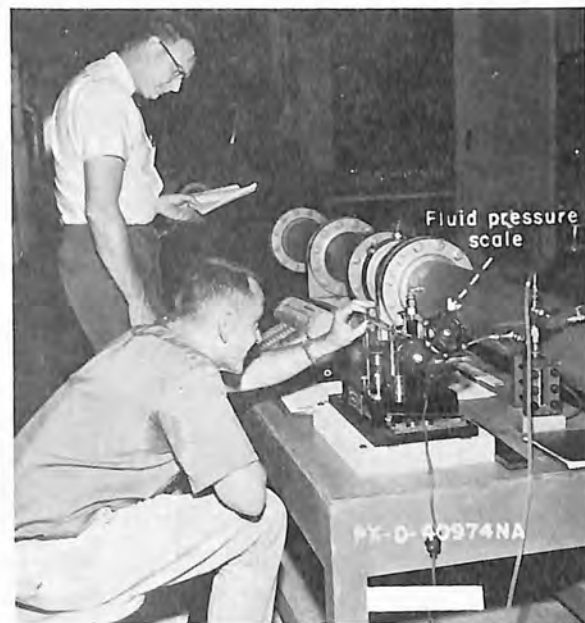
C. Pressure head in the pump discharge line was measured with a 300 psi capacity, fluid pressure scale.
