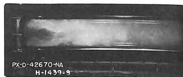
A. Moderately heavy cavitation - K = 0.54 H_T = 145 feet, H_2 = 33 feet
