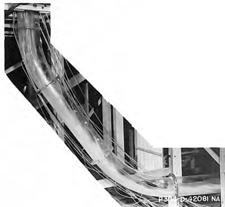
B. Flow in the Bends and Inclined Shaft
