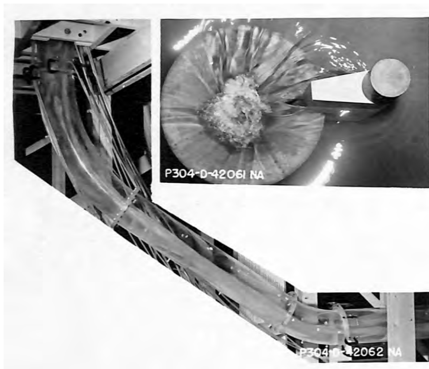
A. Smooth Condition Corresponding to High Point of Boil
