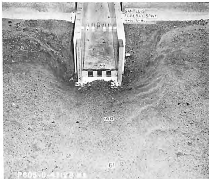
C. 900 cfs T.W. Elev. 165.25 D. Erosion after 2 hours of model operation at 3,250 cfs.
