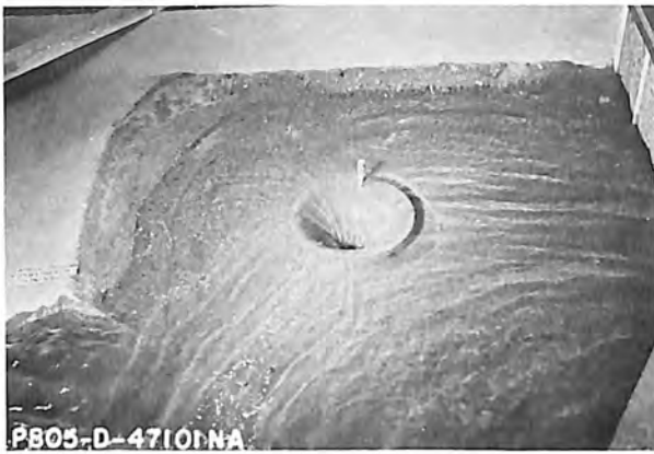
A. 3,250 cfs with wind-generated waves.
