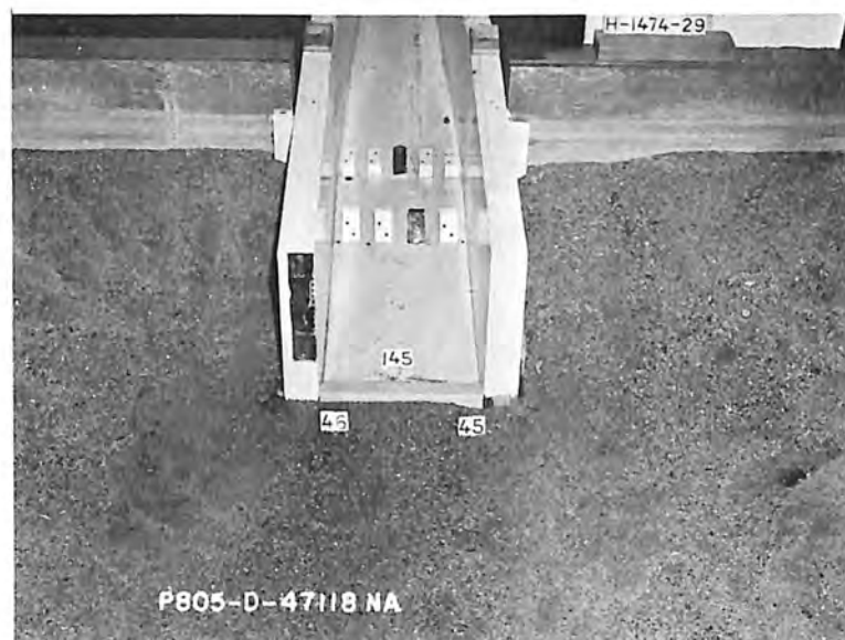
B. Erosion after 2 hours of model operation at 3,600 cfs.
