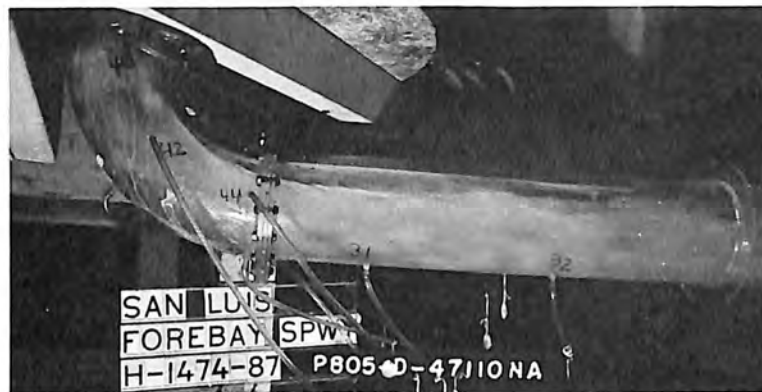
B. 3,250 cfs with reservoir waves.
