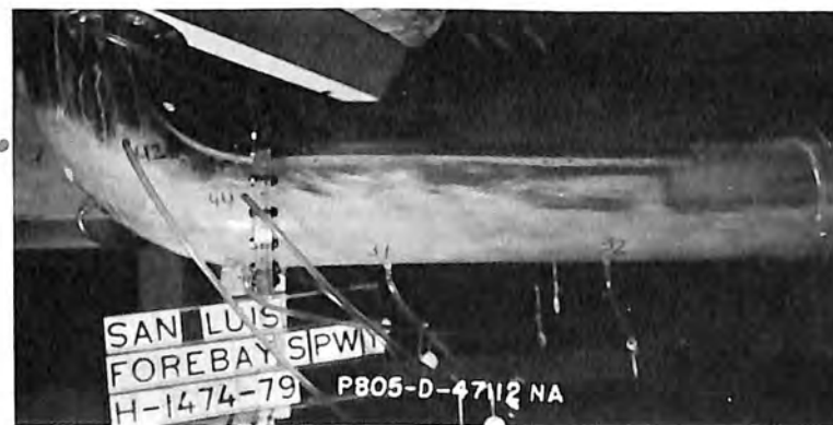
D. 1,500 cfs with reservoir waves.
