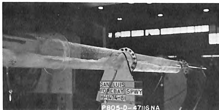
D. 1,500 cfs with reservoir waves.
