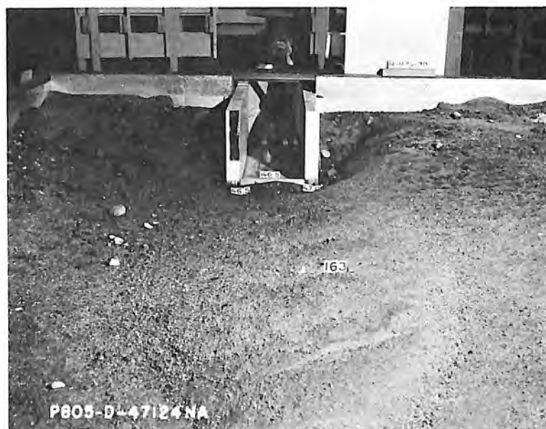
B. Erosion after 2 hours of model operation at 3,600 cfs.
