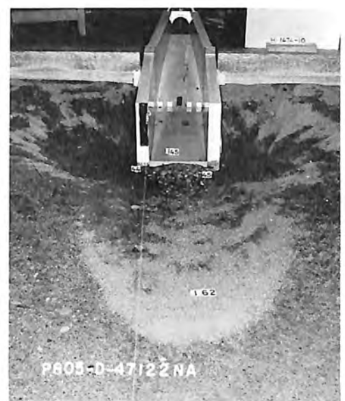
D. Erosion after 2 hours of model operation at 3,600 cfs.
