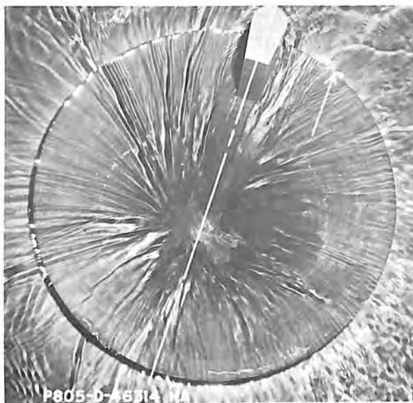
C. and D. Piers on crest with simulated wind waves in the reservoir.
