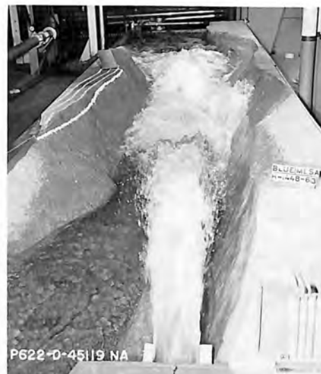
D. Spillway 33,700 cfs Outlet works 5,100 cfs
