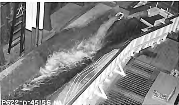
C. Spillway--15,500 cfs
