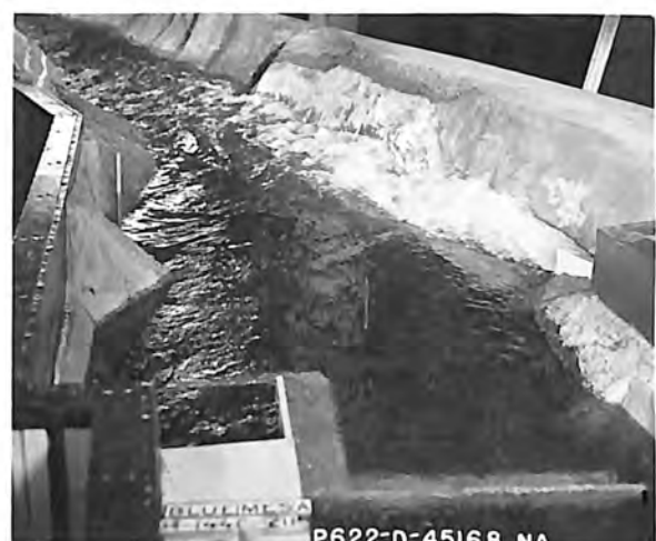
D. 5,500 cfs spillway 5,100 cfs outlet works 3,080 cfs powerplant
