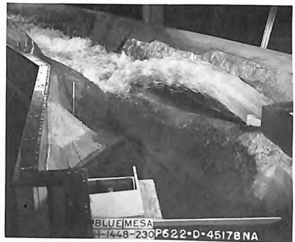
D. 28,000 cfs spillway 5,100 cfs outlet works
