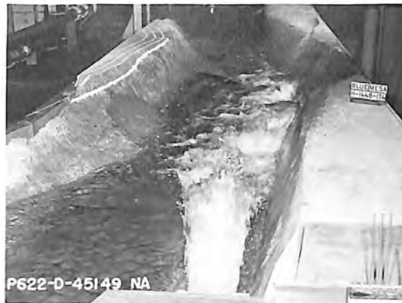
A. Both spillway gates open 5 feet
