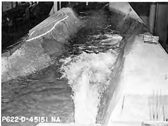
B. Left gate closed, right gate full open
