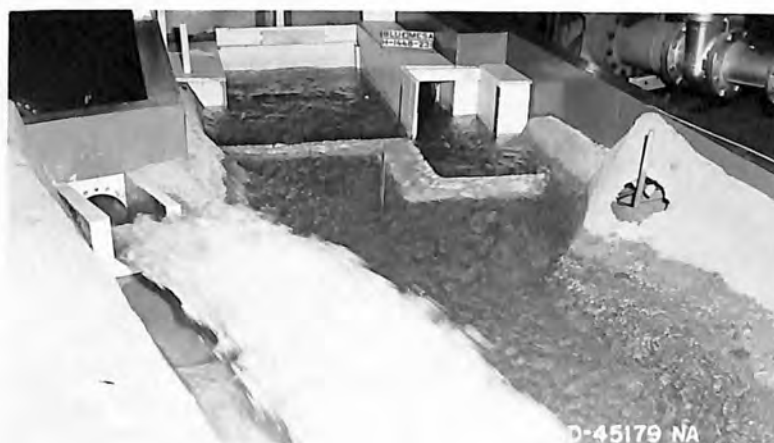
C. 15,500 cfs spillway 5,100 cfs outlet works 3,080 cfs powerplant
