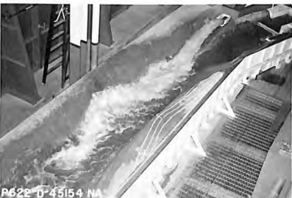
G. Spillway--21,500 cfs Outlet works--5,100 cfs
