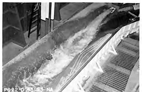
H. Spillway--28,000 cfs Outlet works--5,100 cfs
