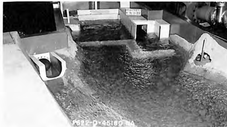
C. 5,100 cfs outlet works 3,080 cfs powerplant
