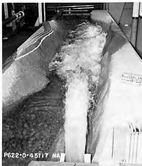
C. Spillway 25,250 cfs Outlet works 5,100 cfs
