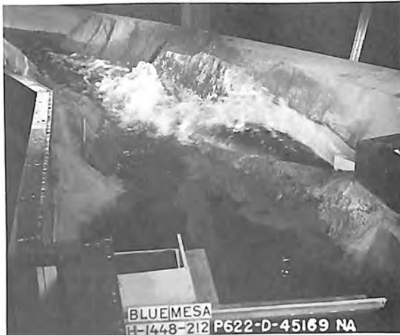
A. 9,500 cfs spillway 5,100 cfs outlet works 3,080 cfs powerplant
