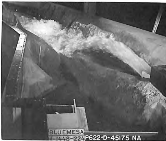
C. 21,500 cfs spillway 5,100 cfs outlet works
