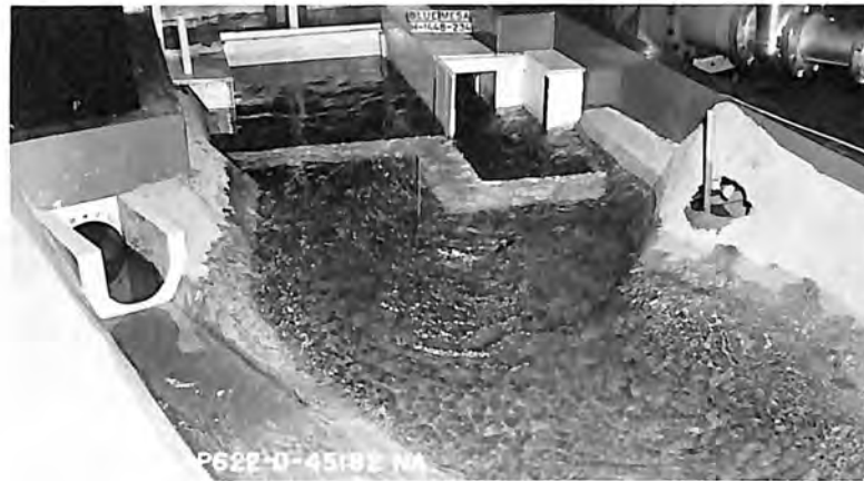
B. 5,100 cfs outlet works
