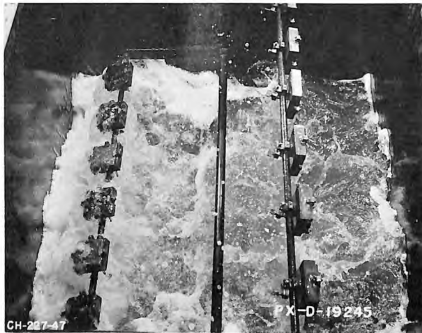
(b) Interior of wave action machine showing turbulent water action
