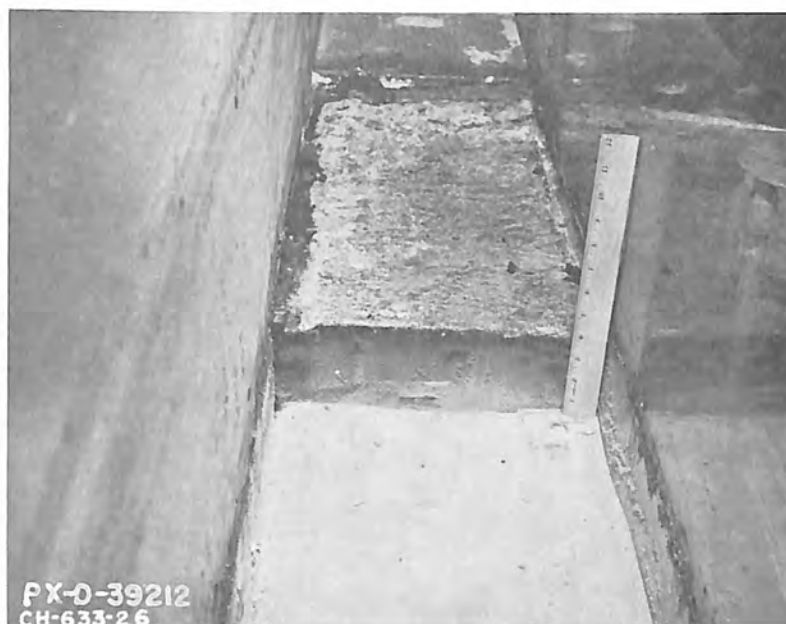
(a) View showing 4-inch depth of soil penetrated by cationic asphalt emulsion sealant
