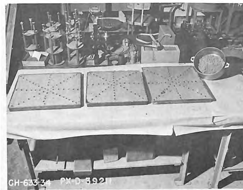
(b) Pans of the mixed sealant-treated soil where small cylindrical specimens were removed for obtaining representative samples for laboratory testing
