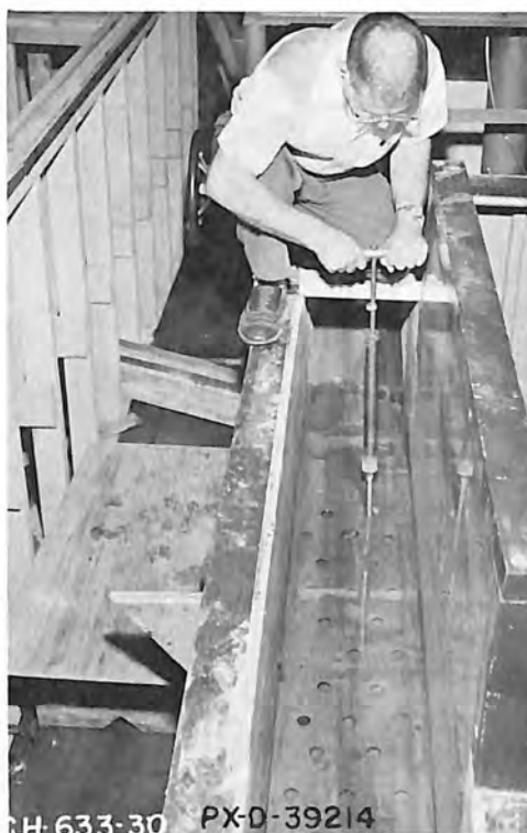
(b) Puncturing surface seal by use of a soil penetration resistance tester with a 1 square inch needle
