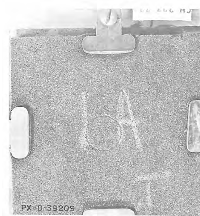
(a) Test specimen molded from asphalt emulsion impregnated sand obtained at surface of test flume
