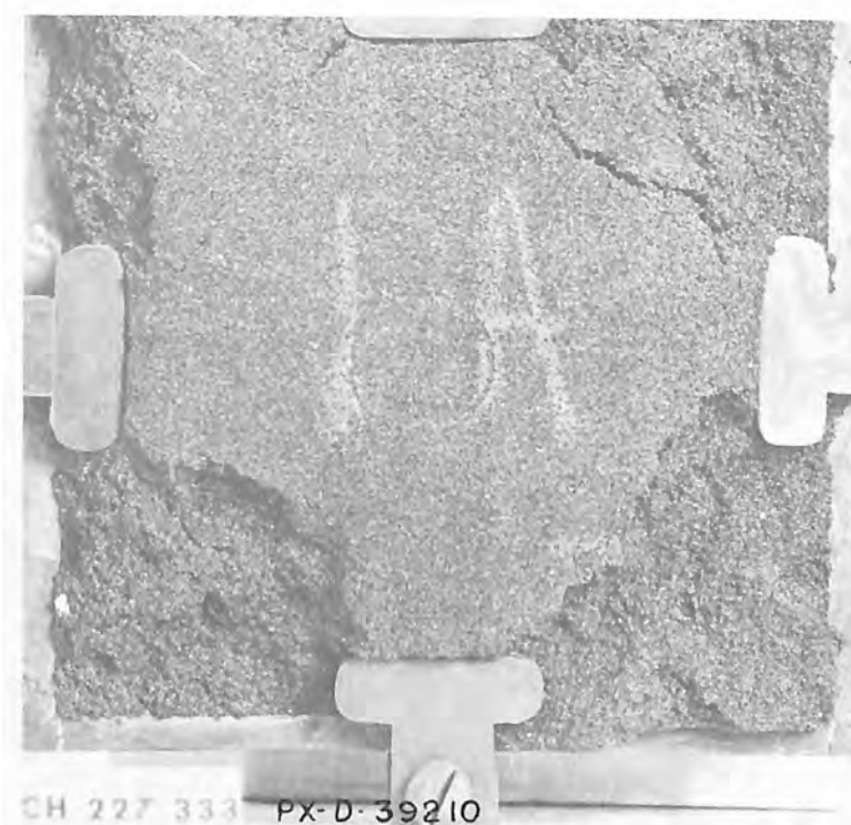
(b) Appearance of test specimen after being subjected to 40,800 blows of wave action
