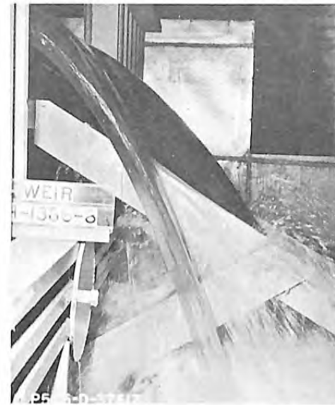
C. Head = 1.7 feet Discharge = 12 cfs
