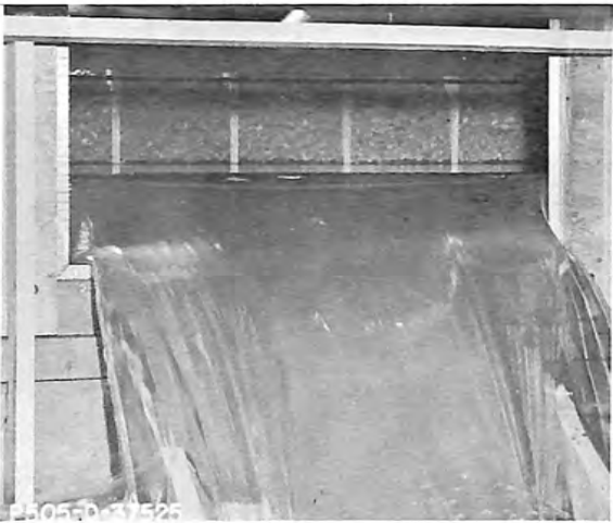
B. Head = 1.7 feet Discharge = 12 cfs
