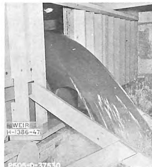
C. Head = 1.9 feet Discharge = 9.8 cfs
