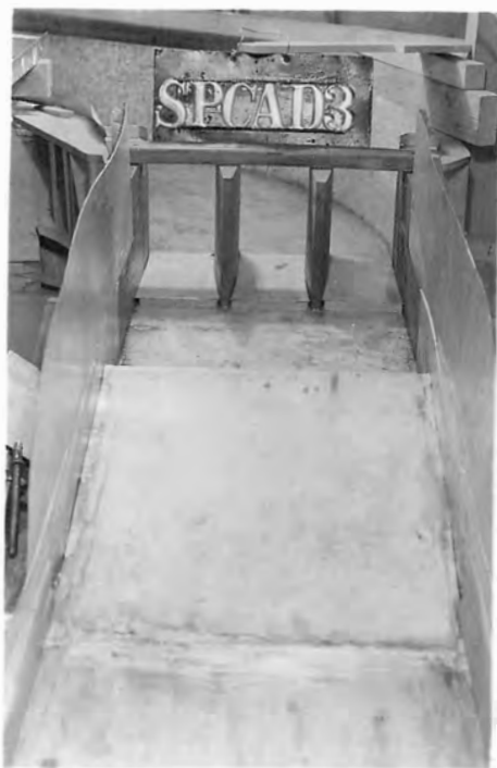
A. ALTERATION TO PRODUCE HYDRAULIC JUMP.
