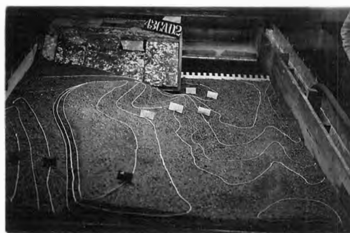
D. BED AFTER ONE HOUR RUN, SAND HAS HAD COARSE GRAINS SIEVED OUT.
