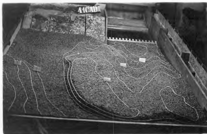
C. BED AFTER RUN, STEPPED APRON 7.9 FEET HIGH.
