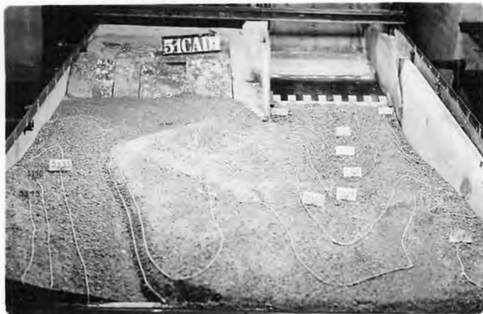
C. BED AFTER ONE HOUR RUN AT 55,000 SECOND-FEET; SILL WITH END BLOCKS.
