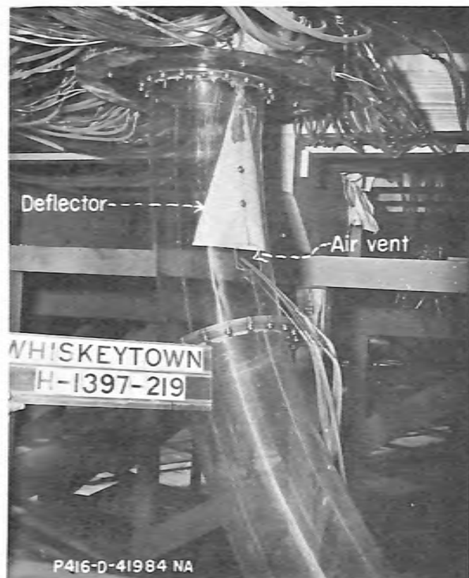
A. Deflector and air vent. Piezometer tubes through air vent extend to the crest piers.
