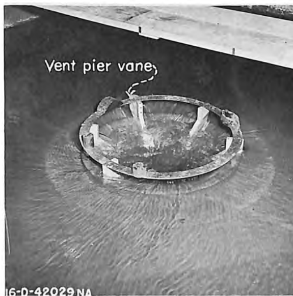
B. Five pier vanes including one with vent intake (28,780 cfs).
