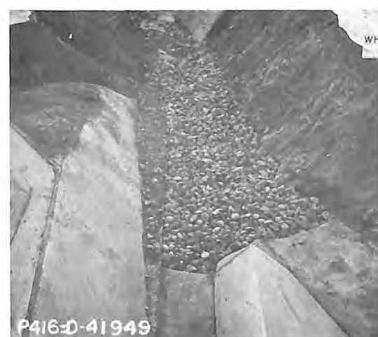
D. Streambed before each test. 1-1/2" gravel.
