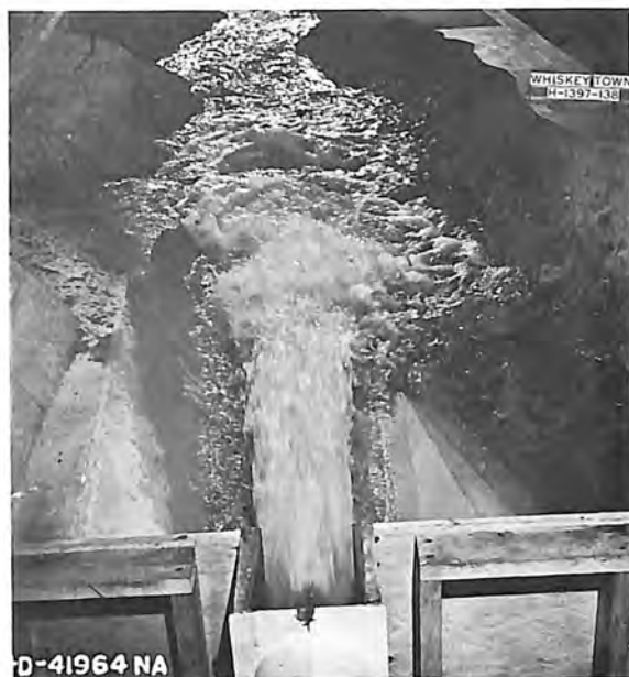
B. 7,125 cfs - Tailwater elevation 959.9
