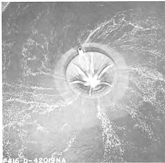
A. Boil forms in throat 27,000 cfs, Res. El. 1218.7.
