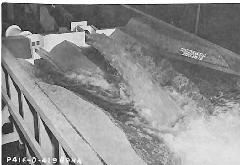
B. Spillway - 21,375 cfs Outlet works - 1,230 cfs
