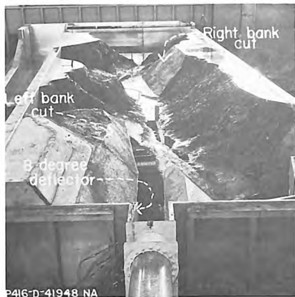
A. 25-degree flip bucket with an 8-degree left wall deflector plus a left bank cut and a right bank cut.
