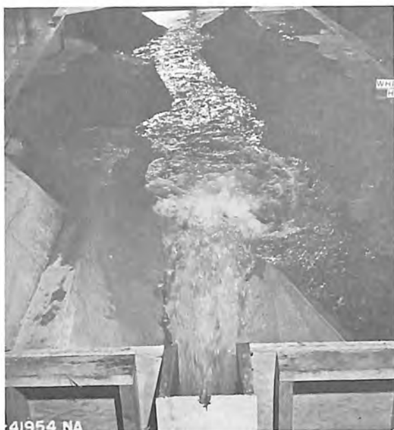
A. 3,560 cfs - Tailwater elevation 956.2
