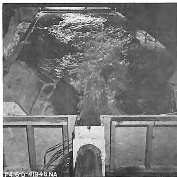
C. 28,780 cfs - Normal tailwater plus 10 feet.
