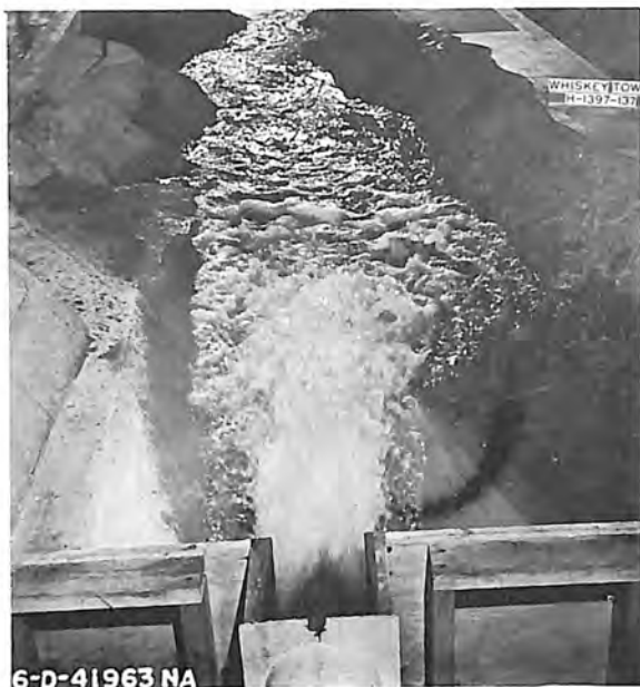
A. 3,560 cfs - Tailwater elevation 956.2
