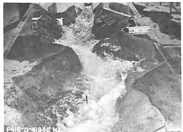
C. 21,375 cfs--Tailwater Elevation 970.0
