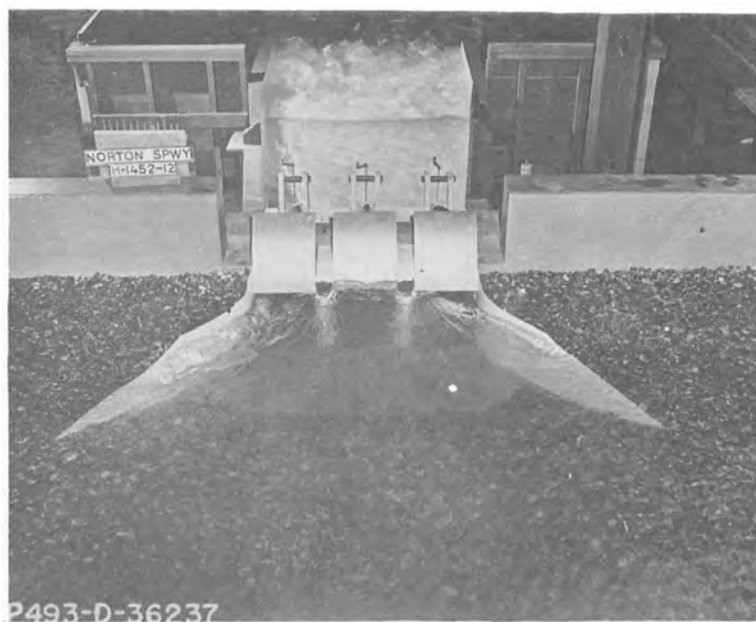
B. Flow at spillway approach. Preliminary piers, recommended. Trunnion location.
