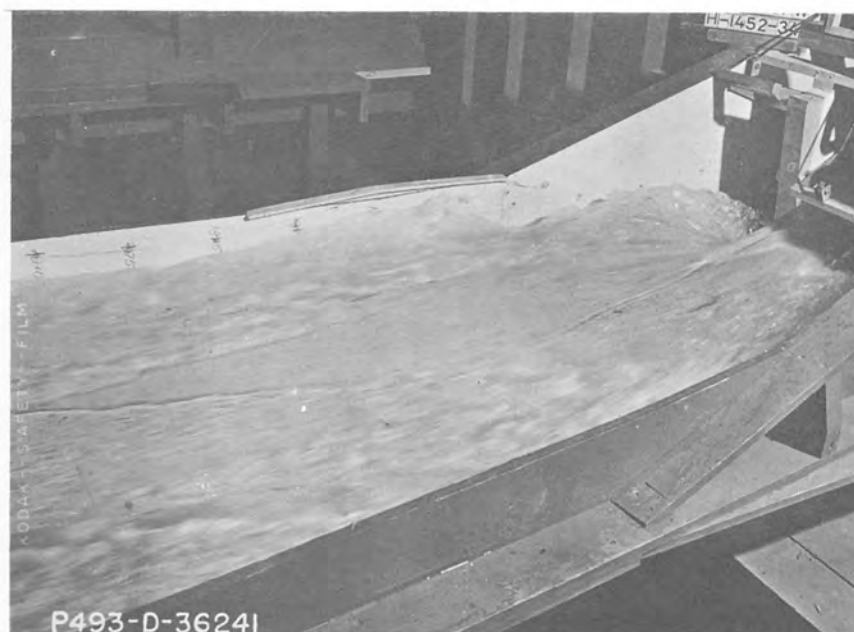
With coping strip on sidewall.
